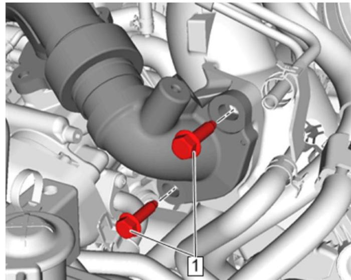
26. Remove the **13mm (#3)** and **10mm (#4)** bolts from the intake manifold and move the radiator surge tank inlet hose aside.
