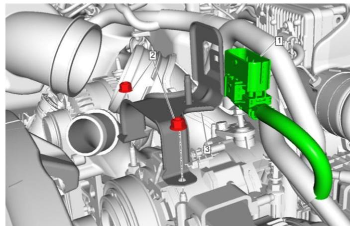
10. Remove the two (2) 13mm nuts, then remove the bracket.
