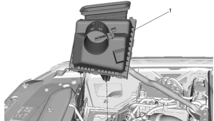
40. Reinstall the air cleaner assembly to its retainers and reconnect the electrical connector.
