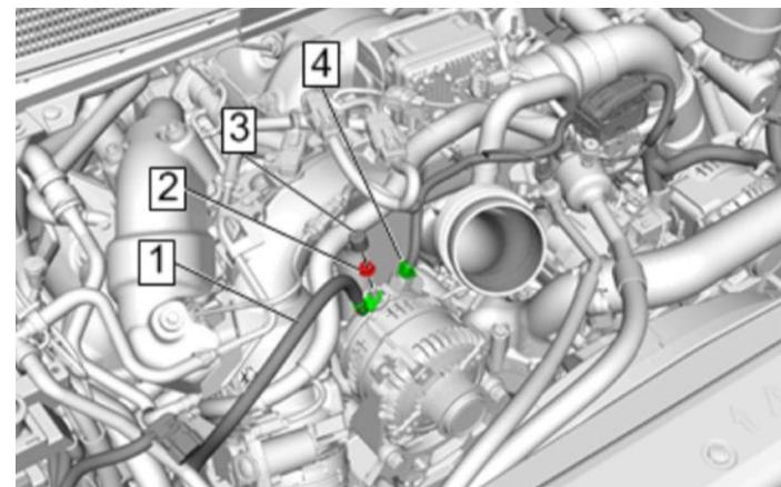
39. Reconnect the alternator electrical connectors.
