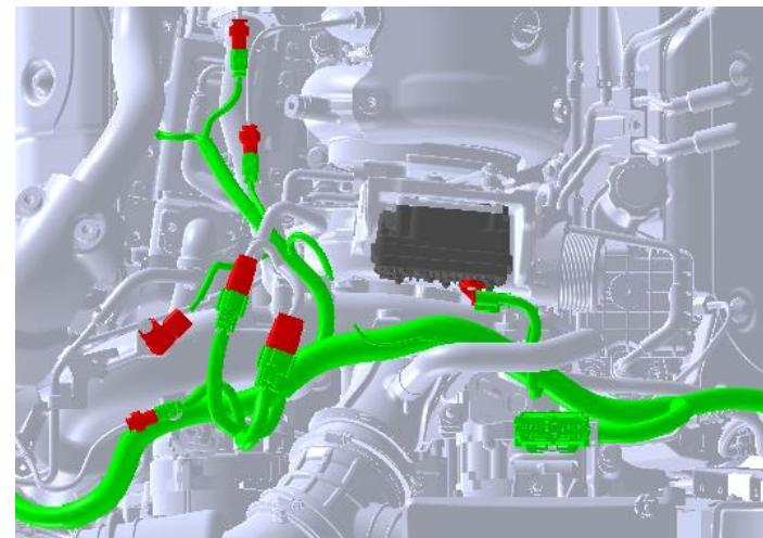
38. Reconnect the engine wiring harness.
