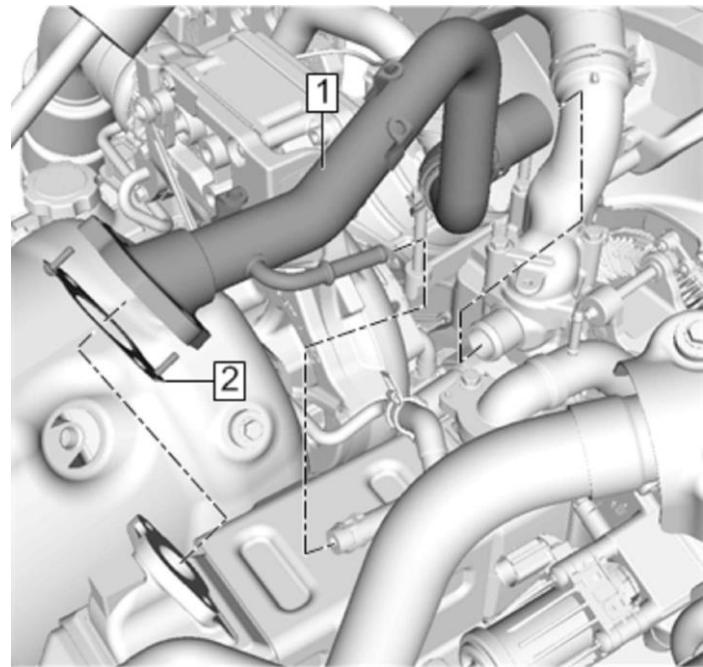
34. Unplug and remove the exhaust temperature sensor (#2) using a **17mm** flare nut wrench.
