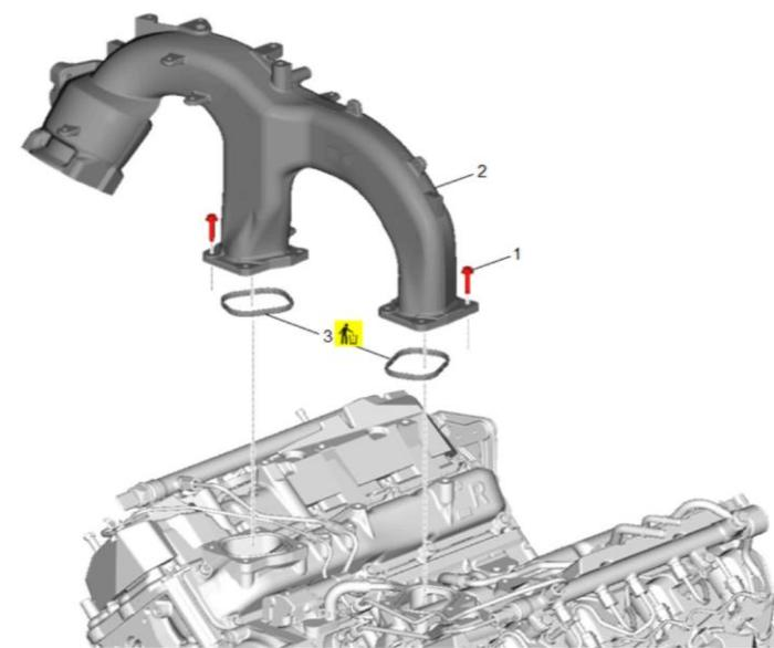
28. Remove the upper intake manifold (#2).
