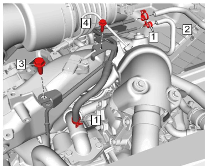
27. Remove the **eight (8) 10mm** upper intake manifold bolts (#1).
