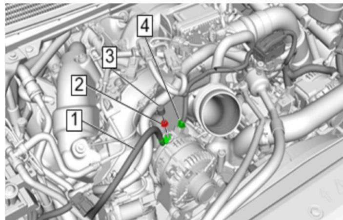
9. Remove the electrical connector (#1) from the bracket (#3).
