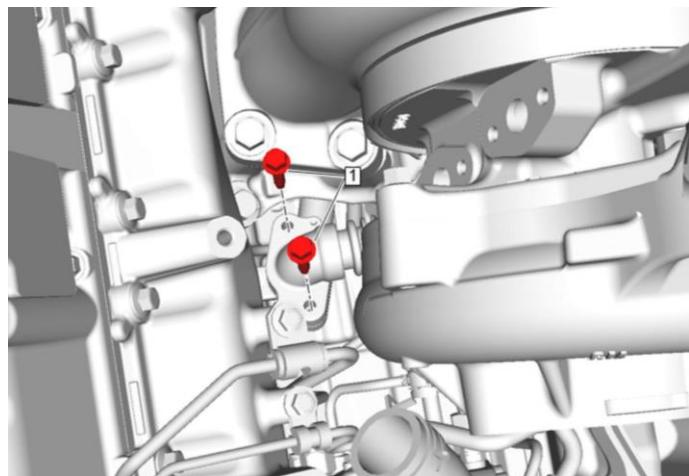
42. Remove the **four (4) 13mm** exhaust front bracket bolts (#1) from the back of the catalytic converter and remove the exhaust front bracket (#2).
