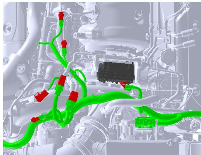
11. Disconnect and reposition the wiring harness as necessary.
