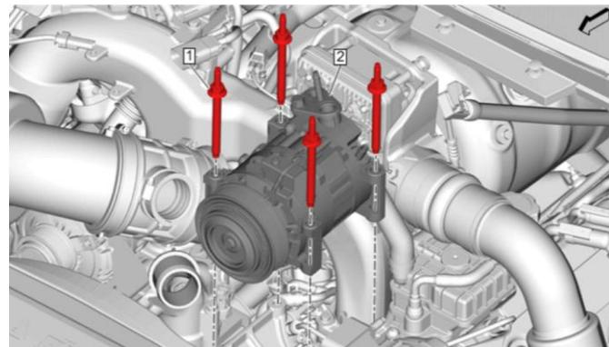
19. Remove the **four (4) 15mm** stud bolts (#1) and move the AC compressor (#2) aside.
