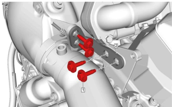
43. Remove the turbo exhaust band clamp (#1) using an **11mm** socket.
