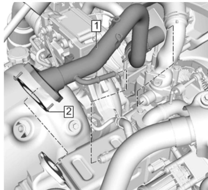
16. Secure the EGR coolant return pipe with **two (2) 10mm bolts (#4)**.
