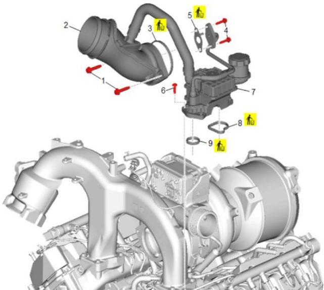
24. Remove the **three (3) 10mm** exhaust gas recirculation valve pipe heat shield bolts (#1) and remove the EGR valve pipe heat shield.
