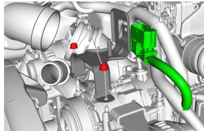
37. Reconnect the electrical connector (#1) to the bracket.
