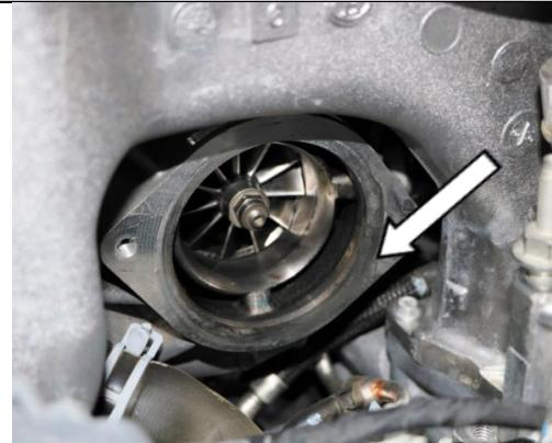
Use very small amount of grease to lubricate the O-ring groove and place the O-ring (FT-920158634) into it as shown. Avoid petroleum or synthetic lubricant which may damage the O-ring
