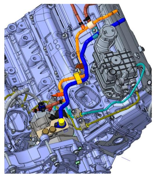
u. Reconnect electrical connector at pump – Inlet Metering Valve in different position on pump, but reuses OE connector and wiring, no adapter/extension needed
