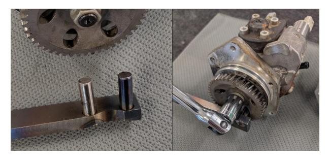
d. Install a **NEW** pump drive gear onto the DCR pump and torque to 48 lb ft (65 Nm) using the gear holding tool and the used nut from the previous step. **Note:** the DCR pump has no key and is normal. Timing the pump to the engine is not required
