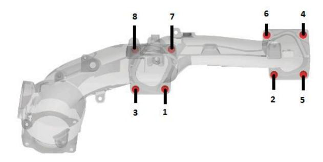
ii. Thermostat housing tightening sequence
