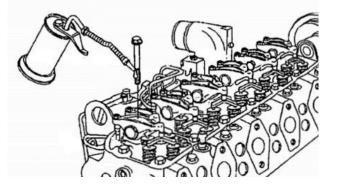
**STEP 4:** Tighten the cylinder head cap screws in the sequence illustrated.
