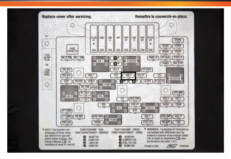
Insert the original fuse from the fuse block into the relay tap below the 5A fuse that is provided in the fuse tap. Both fuses are required for the tap and existing circuit to function properly.
