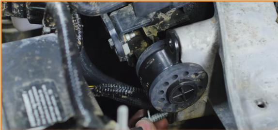
12. Separate the airbag sensor from the upper support bar. Simply remove the screw. DO NOT disconnect the harness. (1x 8mm bolts)
