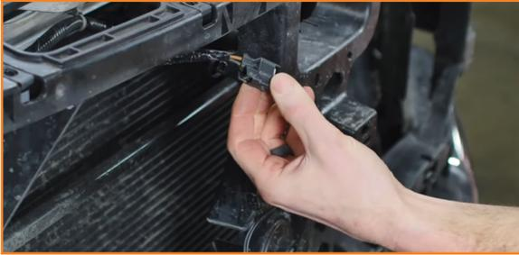
9. Detach all the components on the upper support bar. (4x 10mm bolts)
