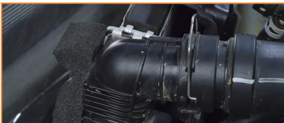
26. Slide the overflow hose off the radiator. (1x spring clamp)
