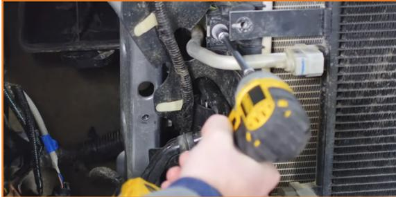
19. Disconnect the shrouding from the radiator and secondary radiator.
