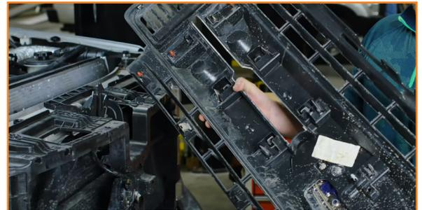
4. Remove the bolts that secure the headlights. There is one bolt on top, two on the front, and one underneath. (6x 10mm bolts, 2x 8mm bolts)
