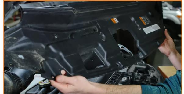
3. Remove the bolts at the top of the grille. Pull the grille off the front of the truck. Note the orange tabs on the inside for when you must reinstall the grille. (8x 10mm bolts)
