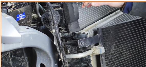
22. Release the quick-disconnect at the bottom of the secondary radiator. (1x spring clip)
