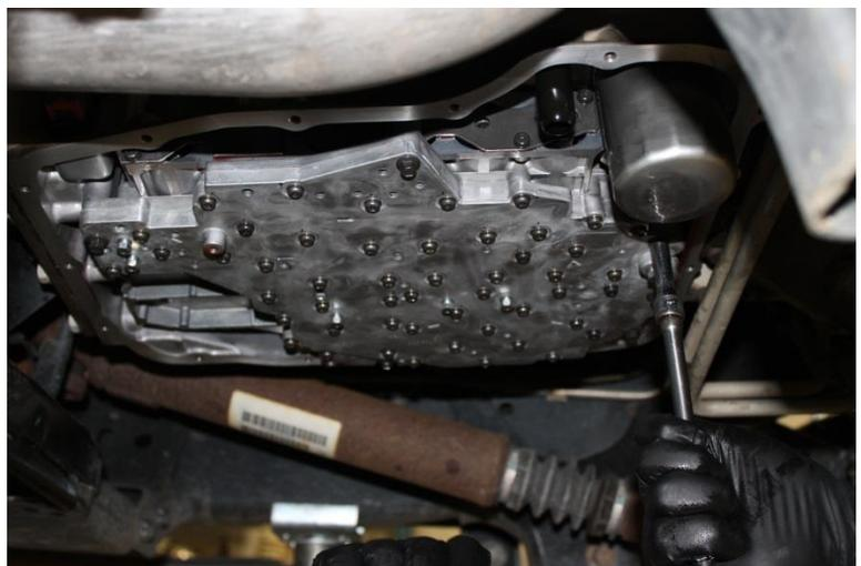
32. If desired, install new filter(s). Otherwise, reinstall the filter/pickup assembly. Torque to 50 in/lbs.
