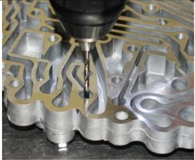
20. Thoroughly remove any burrs and clean all shavings from the valve body. It is imperative that no contaminants are left as they may cause transmission damage.
