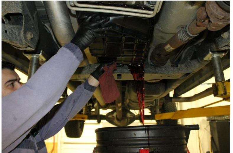
10. Remove transmission filter by removing the one T25 Torx screw.
