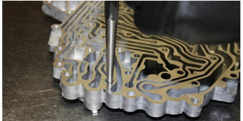
19. Drill hole with 1/8" drill bit.
