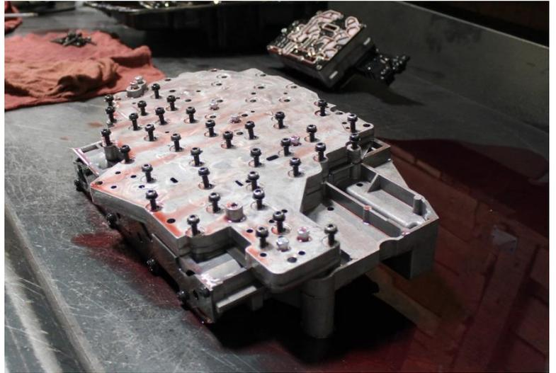
15. Carefully separate the two halves of the valve body. Separate as shown in pictures – *do not invert the larger (top) portion as it contains plastic check balls*. The two halves will have to be wiggled apart as the alignment dowels will be holding them together.
