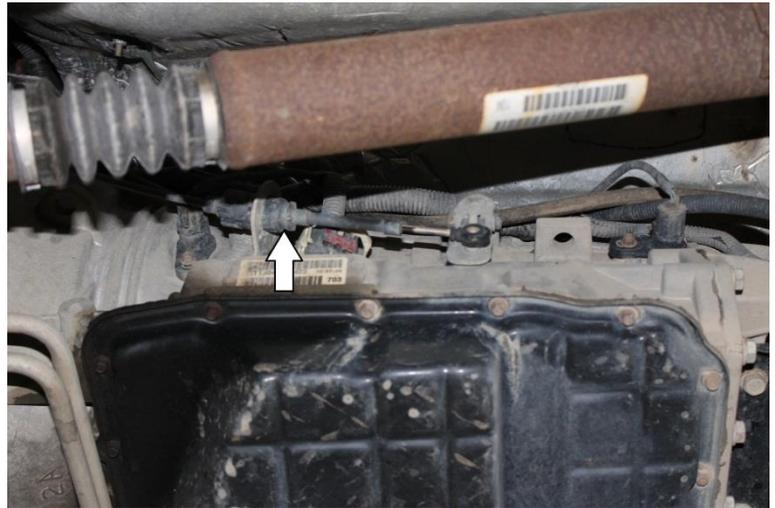
6. To remove connector, push red tab (1) downwards. Then, press the black tab (2) which will allow the white handle (3) to be rotated downwards, releasing the connector from the transmission.
