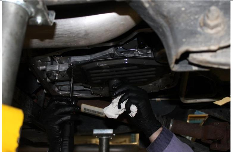
33. Place the supplied gasket on the transmission pan. Hold pan below transmission and install attaching screws. Torque the pan screws to 105 in/lbs.
