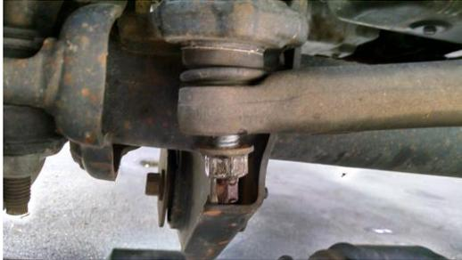
3. Remove the stock bolt and nut from the trac-bar frame mount. Remove the stock trac-bar. **Note:** Tie-downs attached to the axle and frame may be necessary to prevent the axle from shifting after removing the bar, this will aid when installing the new bar.
