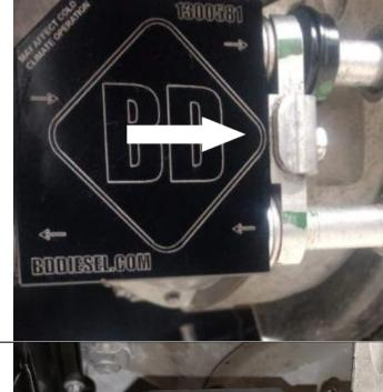
Reinstall both transmission cooler lines in to threaded end of the block, wiggle the lines and nut to start the threads. Tighten nuts 24 lb-ft.
