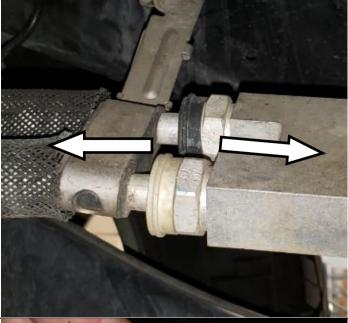
The original thermostat housing should now be removed. Clean the ends of the lines if needed to prevent debris contamination upon reassembly.
