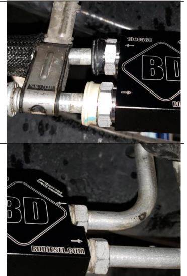
Inspect original O-ring on the tube, replace with supplied viton O-ring (1453153) if it is damaged.
