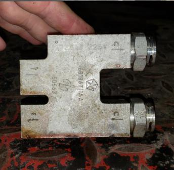
Put quick connect fitting (1300579) on thermal by pass block (1300580) using 1" and 24mm open wrench.
