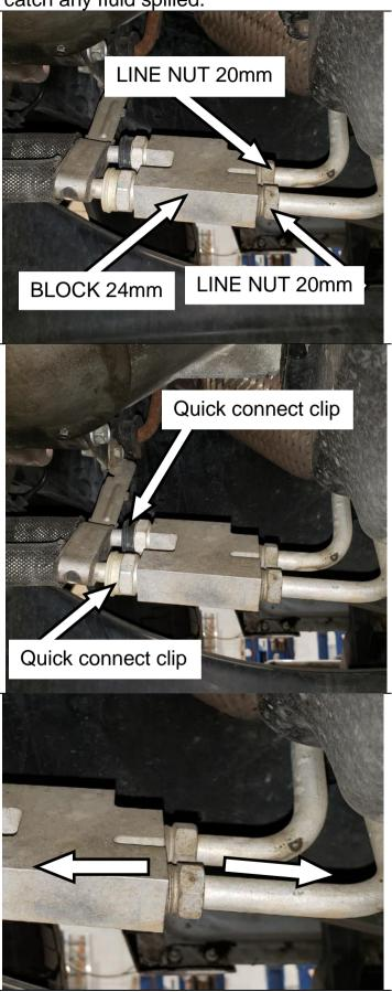
Pull cooler bypass block off of the quick connect lines
