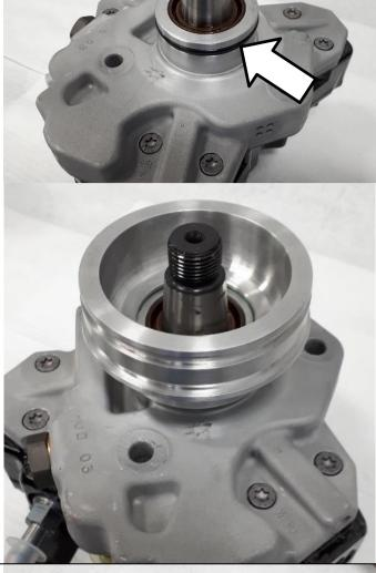
Install supplied gear onto pump shaft, and secure in place with supplied flat washer and nut.
