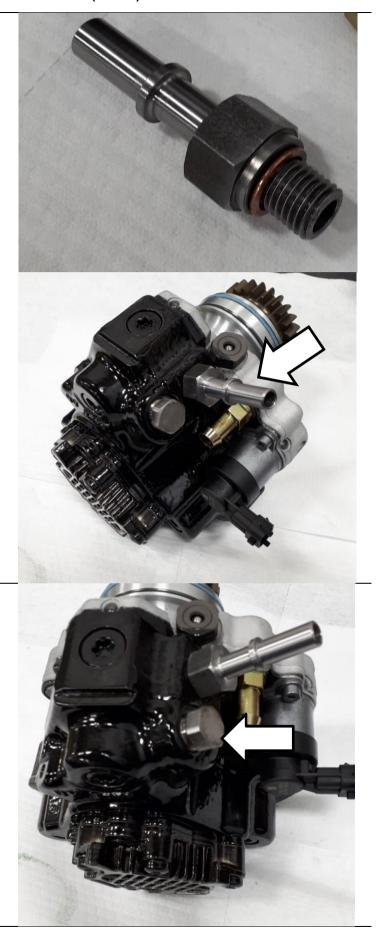
Remove High-Pressure plug from back of CP3 pump, located adjacent to the return fitting and OEM High-Pressure outlet.
