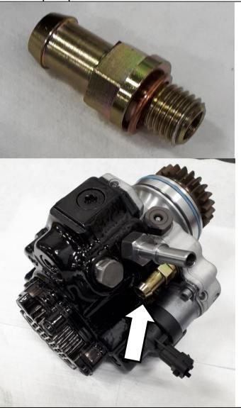
Remove OEM return fitting, and install supplied Quick-Connect fitting.
