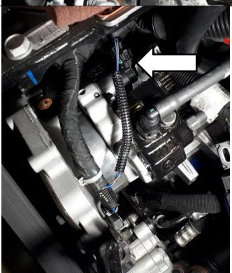
Ensure wiring is all secured and won't rub on hard parts.
