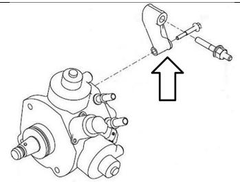
Remove three (3) mounting nuts holding CP4 pump to engine, and remove pump by pulling it towards rear of the truck.
