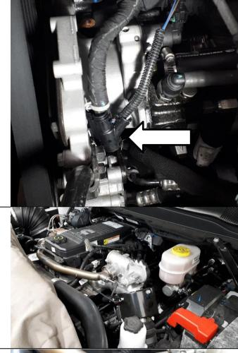
Reinstall intake horn, EGR cross over pipe and associated parts removed earlier.
