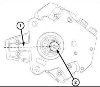
Install CP3 pump onto engine, keeping the alignment from the previous step.
