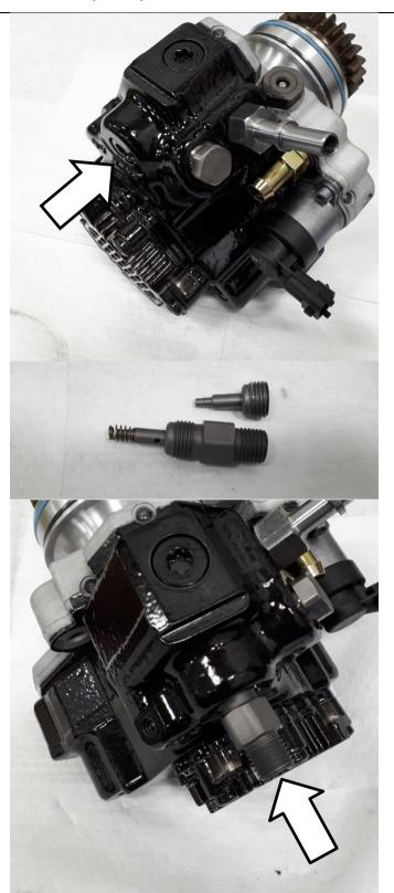
Ensure CP3 pump o-ring is installed, and install pump collar onto the front of the pump.
