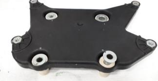
Remove standoffs and grommets from OEM ECM bracket.
