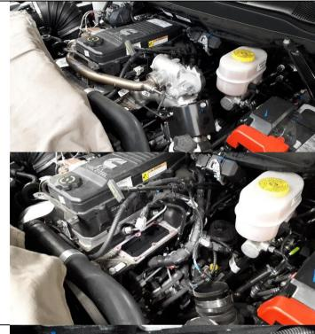
Unplug connector from CP4 pump, and Disconnect Feed and Return quick Connect hoses.
