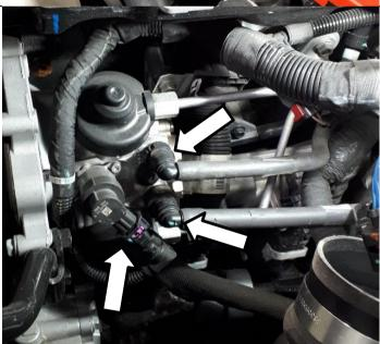
Disconnect high pressure fuel lines from CP4 pump, and Fuel rail. Remove fuel lines from engine.
