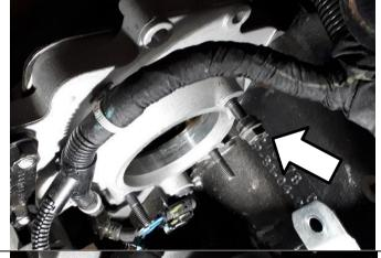
Install supplied adapter plate using three (3) supplied socket head cap screws.
