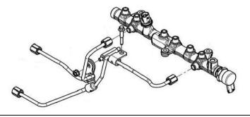
Remove nut from harness support, and remove CP4 support bracket from engine.
