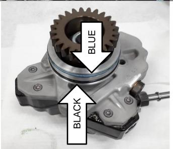
Set the correct timing for the pump as follows.
