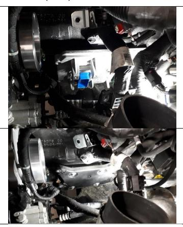
Remove the four (4) bolts retaining the ECM bracket, and remove ECM bracket from the engine.
