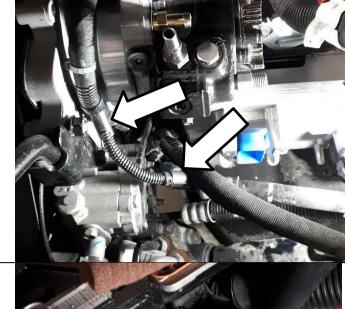
Route connector towards CP3 metering unit, and plug harness into pump.
