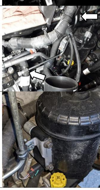
Remove factory loom 'Y'-clip, and both clips attached to the CP4 harness connector.
