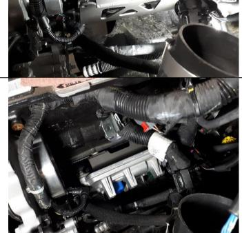
Remove o-rings from CP4 pump collar, and install them onto the collar previously installed on CP3 pump.
