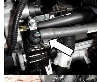
Install supplied High-Pressure fuel line between the CP3 pump and forward open fuel rail feed port.
