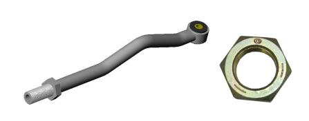
Thread the passenger side track bar section into the threaded connector (1302030-4). The passenger side track bar is Left Hand threaded, so you will need to mate these threads to the left-hand thread of the connector. The left-handed threads should be identified with an "LH".
