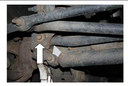
With the factory track bar removed, use a tape measure and measure the length of the factory track bar from the center of the bushing to the center of the bushing.
