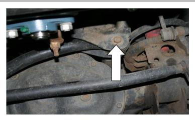
Using the 18mm socket (2003-2012) or 27mm socket (2013-2022) remove the passenger side track-bar bolt. Save the bolt for re-use during installation.
