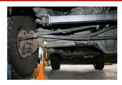
Using an 18mm socket (2003-2012) or 27mm socket (2013-2022) remove the driver's side track-bar bolt. Save the bolt for re-use during installation.
