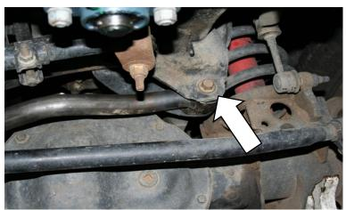
If required perform an alignment on the front end of the vehicle. Adjust the front axle left and right by turning the threaded connector.
