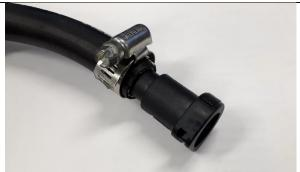
Remove factory feed hose from bottom of fuel bowl, and replace with ½" fuel hose assembled in previous step. Connect hose to CP3 pump inlet fitting with supplied clamp.
