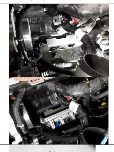
Install CP3 pump onto engine. Install using three (3) supplied flange bolts. Pump will install with the metering unit pointing upwards.
