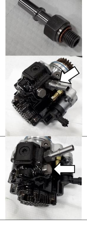
Remove High-Pressure plug from back of CP3 pump, located adjacent to the return fitting and OEM High-Pressure outlet.
