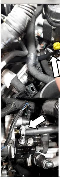
Connect OEM return hose to CP3 pump as shown.
