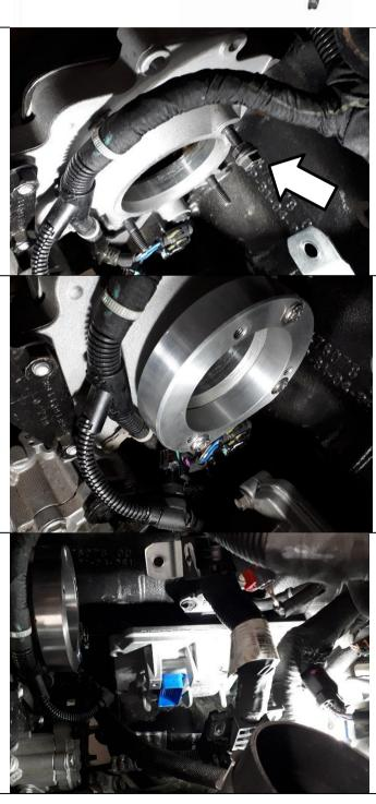
Remove four (4) bolts holding ECM in place, and remove ECM from the engine.
