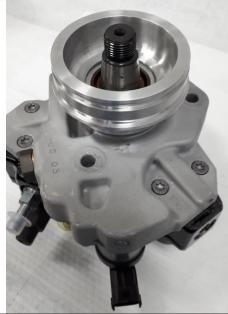
Install supplied gear onto pump shaft, and secure in place with supplied flat washer and nut.
