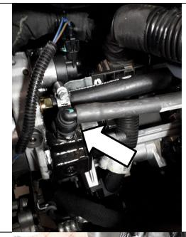
Install supplied High-Pressure fuel line between the CP3 pump and forward open fuel rail feed port.
