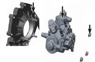
Remove three (3) CP4 mounting studs from engine. Using two (2) CP4 mounting nuts, double nut the stud and unscrew it.
