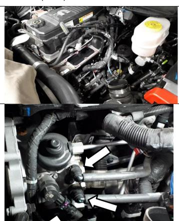
Unplug connector from CP4 pump, and Disconnect Feed and Return quick Connect hoses.
