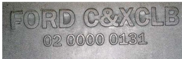
**Note:** *The tank body has the above identification on its top. Please check to be sure the tank is properly identified as the one to fit your vehicle.*
