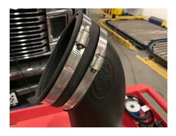
Insert the Intake Tube (T) into the Box Seal (M) located on the Air Box (A). Work the Intake Tube (T) slowly, at the angle shown, until the bead on the Tube is up against the Box Seal (M).
