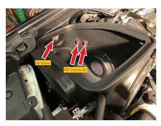
Tighten the screw that was hand tightened in Step 21 to secure the Air Box Bracket (H) to the fender frame.
