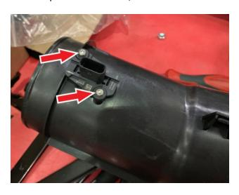
Make sure the stock gasket is on the MAF sensor and place the MAF Mount (V) first and then the MAF Mount Gasket (U) second on to the stock MAF sensor as shown.
