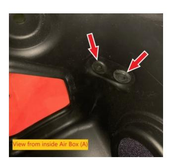
From the inside of the Air Box (A), install Shoulder Bushings (F) into the Grommets (E)
