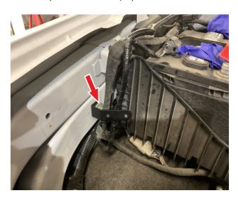
Carefully work the Air Box (A) into the vehicle. The space is tight but carefully move/rotate the box to make space for the grill inlet duct, fender, and coolant reservoir as you lower the Air Box. Once the Air Box is below the fender it will become easy to position the Air Box properly then push down to fully seat the Washer (D) into the stock bottom box grommet shown in Step 12. The AirBox should snap into the grommet.
