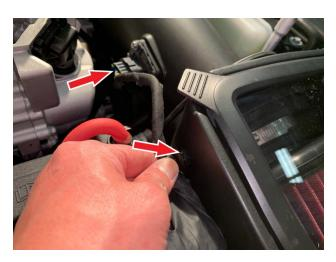
After the batteries have been disconnected for at least 2 hours, reconnect the positive battery terminal on the passenger side first and torque the terminal clamp nut to factory specifications, 80 lb-in (9 Nm), and place the cover over the terminal. Then reconnect the negative terminals on both batteries and torque the terminal clamp nut to factory specifications, 80 lb-in (9 Nm).
