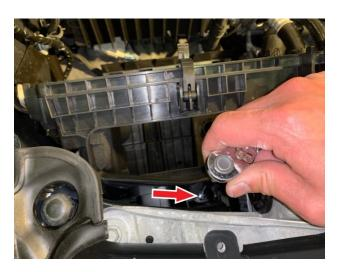
Firmly but carefully rock and lift the intake box free from the lower grommet and free the side rubber bushings from the side saddle bracket. Remove the intake box from the vehicle.
