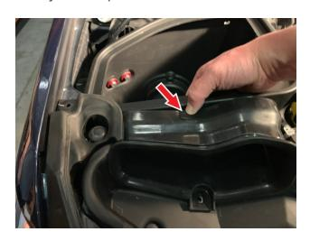
Secure the Air Box Inlet (P) onto the vehicle with the push in rivet removed in Step 8. Make sure the push in rivet is fully inserted and the center stem pushed all the way down.
