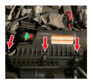
Carefully remove the stock intake filter.
