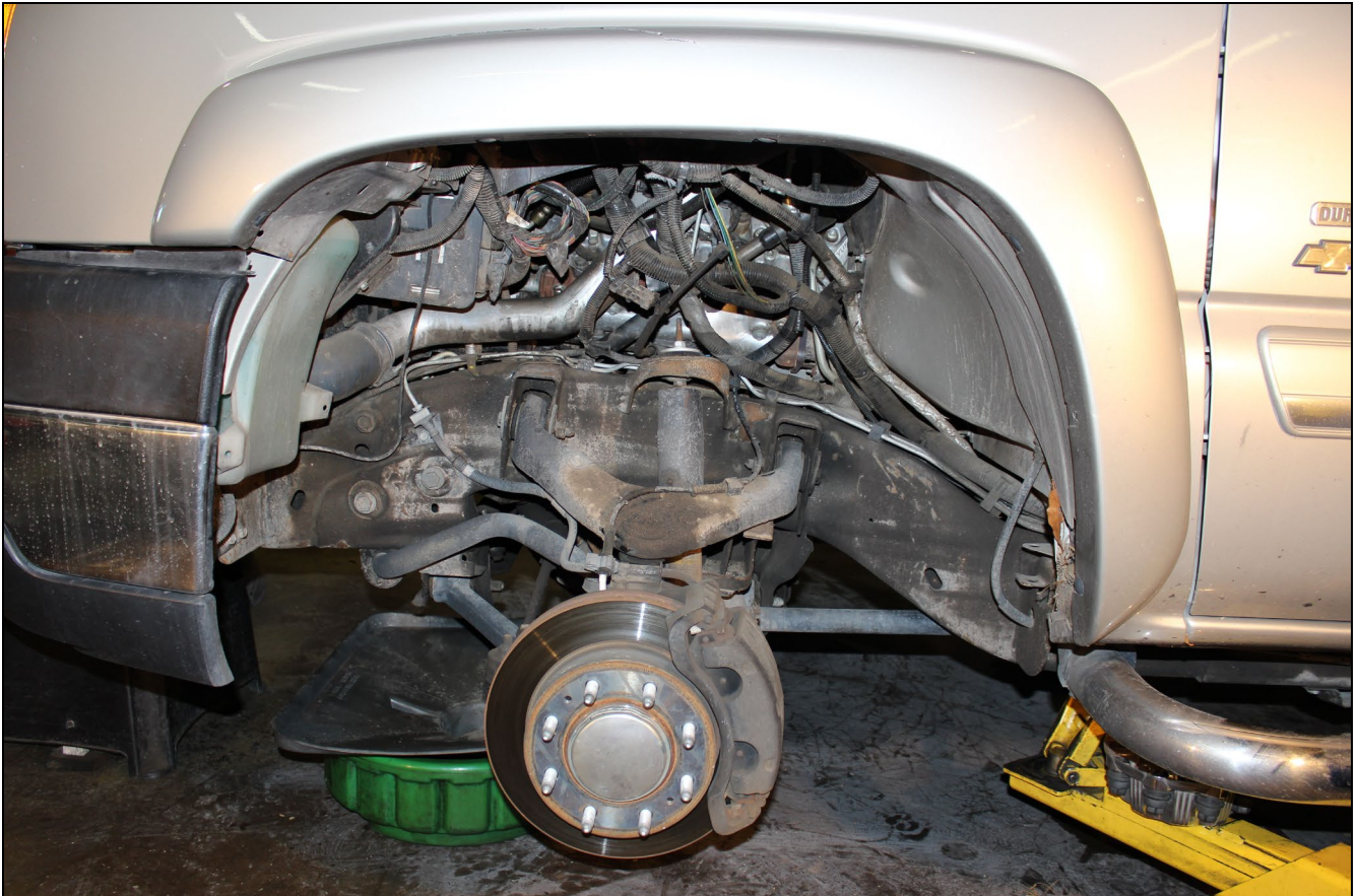
FIGURE 3 – INNER FENDER REMOVED
