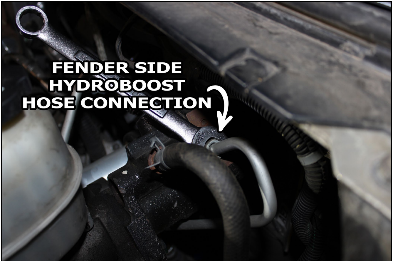
FIGURE 12 – FENDER SIDE HYDROBOOST HOSE/TUBE CONNECTION
