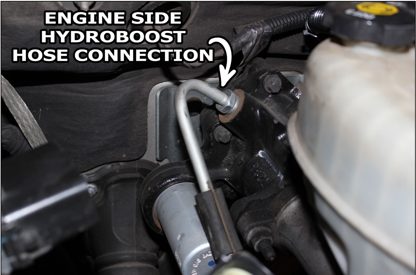
FIGURE 11 – ENGINE SIDE HYDROBOOST HOSE/TUBE CONNECTION
