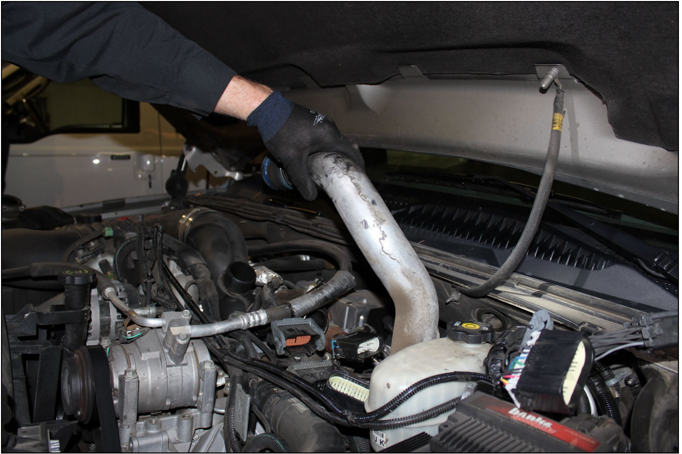
FIGURE 6 – REMOVING THE DRIVER SIDE INTERCOOLER TUBE
