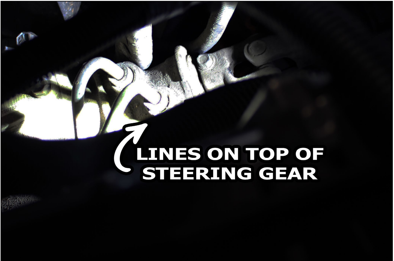
FIGURE 9 – POWER STEERING LINES AT THE STEERING GEAR
