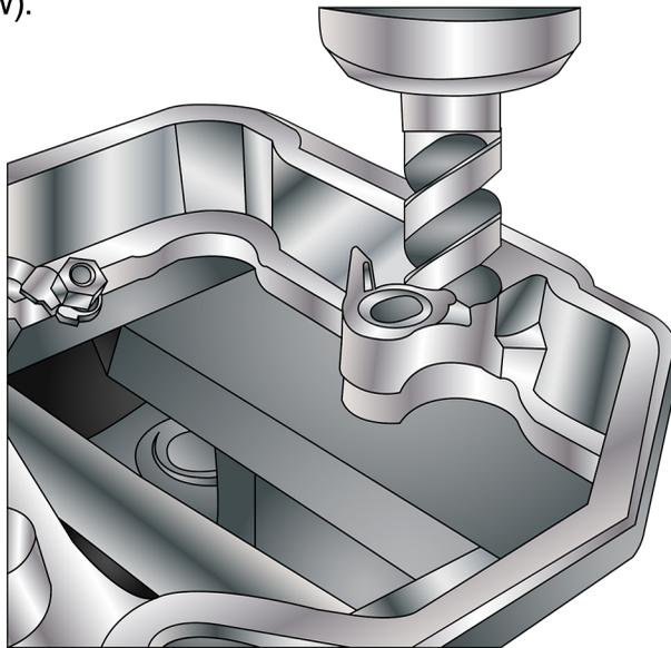
**Remove material as necessary to allow clearance for the stud, nut and washer.**
