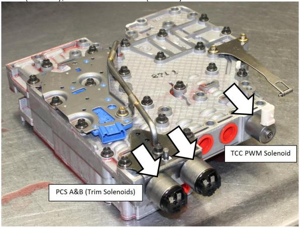
1030471-1030473 – 2004-2010 Allison valve bodies are supplied with four solenoids. Pressure Control A (TRIM A), Pressure Control B (TRIM B), TCC PWM and Main Mod (G Solenoid).
