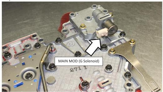
Remove the wiring harness from the stock valve body.
