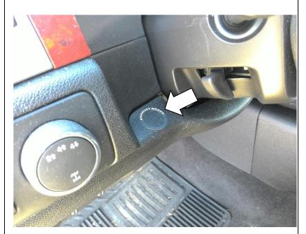
8. Plug the white connector from the VVB harness into the back of the switch and secure wiring with supplied zip ties under the dash.
