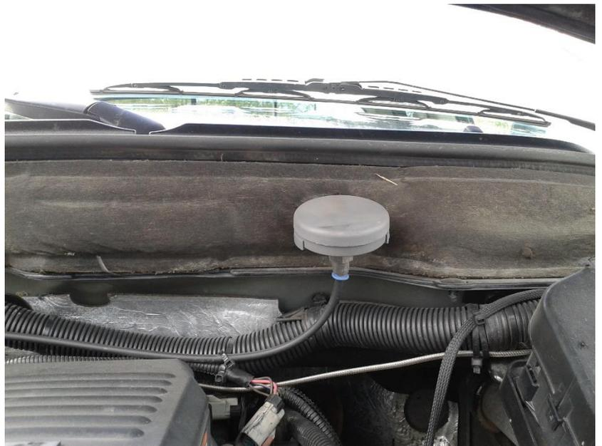
Locate the 1/8" tube from in the air tubing assembly that leads to the brake valve. This will be installed in the output from the air regulator assembly on the bottom of the solenoid. Trim this tube to length and install it in the 1/8" fitting.
