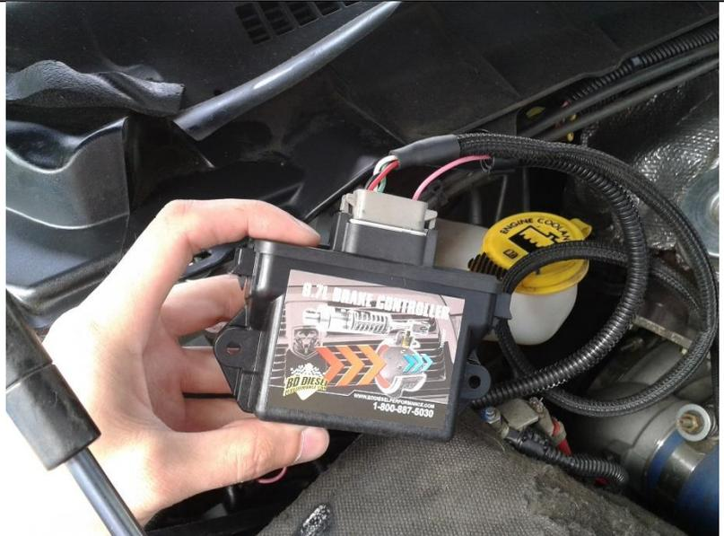
Connect the pink trigger wire from the module harness to the air regulator assembly's pink wire using the pre-installed butt connector.
