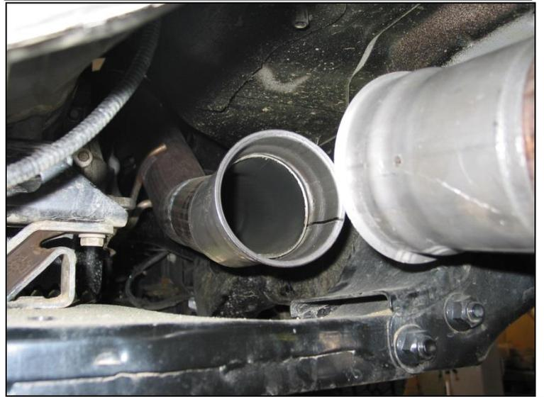
Ensure the exhaust brake and rear exhaust sections are pushed all the way forward on the front pipe so that the front adapter flange is up against the stop that is on top of the front pipe section then WELD the front adapter in place. Install the rear adapter to the pipe using the supplied band clamp.
