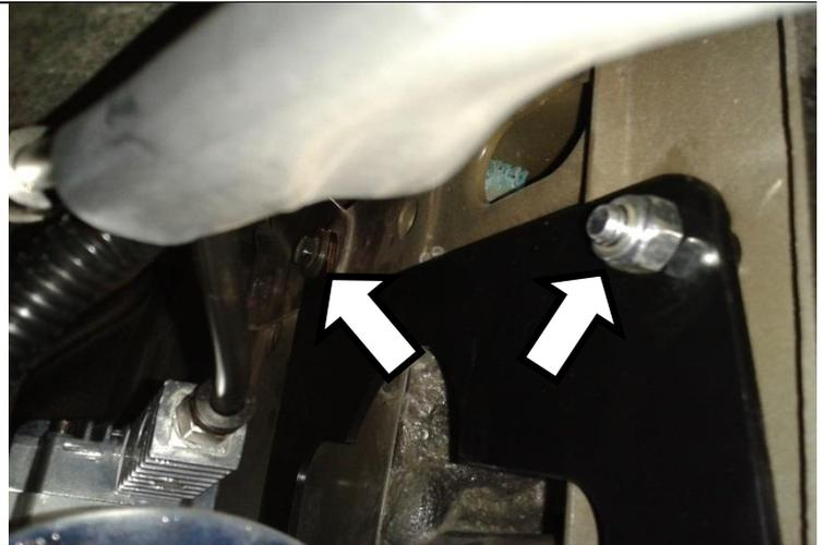
While the fender liner is off, double check that the air tubing assembly installed in the earlier section is well clear of the exhaust pipe, turbocharger and moving suspension components.
