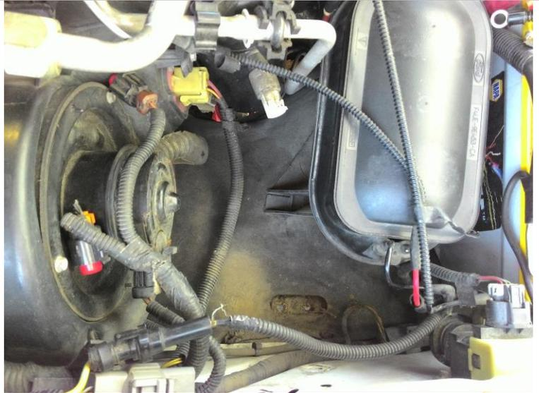
To install the BD compressor, first remove the two 11mm nuts securing the vacuum reservoir to the fender. These are accessed from in the wheel well below the reservoir.
