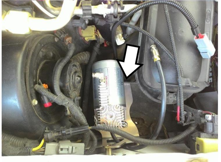
**Note** Disconnecting the AC pressure switch electrical connector and moving the harness out of the way temporarily will make this process easier.
