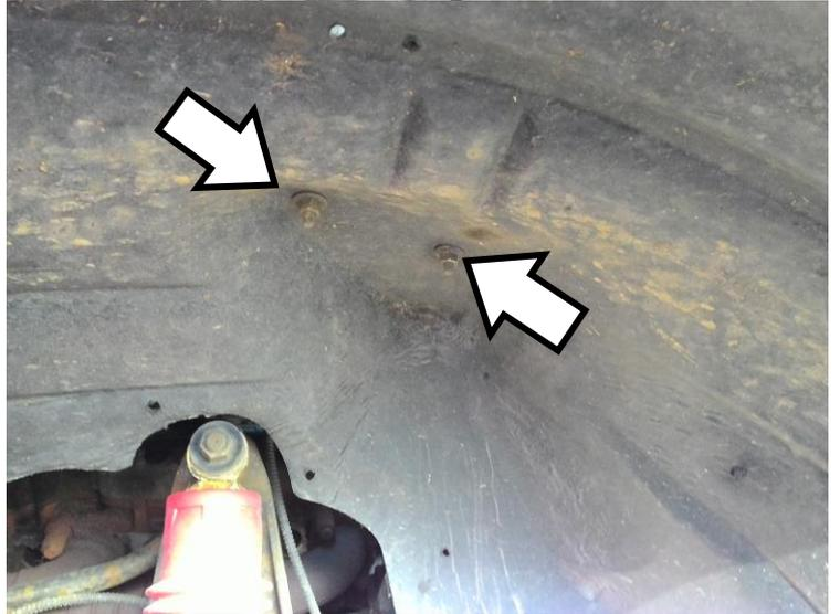
Once the vacuum reservoir is loose, slide the air compressor bracket under the rear mounting stud for the reservoir.
