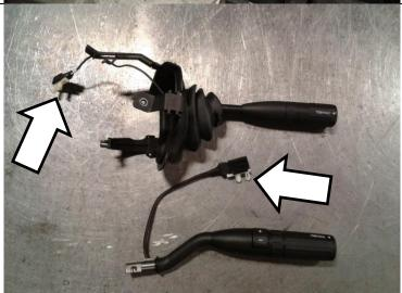
16. Remove the boot from the old shift lever and transfer to the new one. The boot will have to be stretched to fit over the electrical connector.
