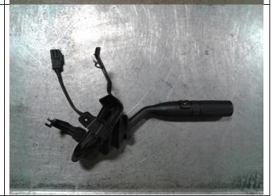
17. Install new shift lever by re-installing T30 securing screw and the two 5.5mm boot attaching screws. Secure the wire with a wire tie to the plastic wire clip such that the wire will not rub or chafe during use.
