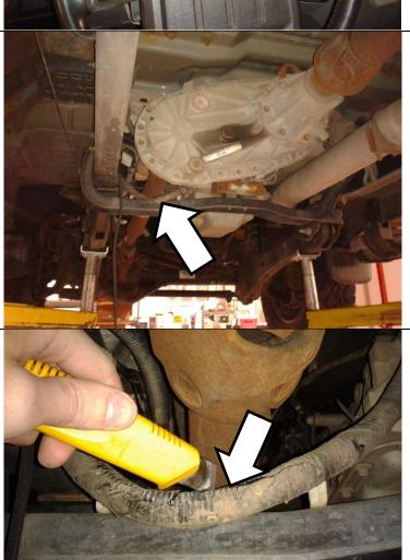
24. Pull wires out of the harness and locate the 20 gauge gray wire with a brown tracer. Use care when locating the wire as there is an 18 gauge wire of the same color for the ISS in this harness.
