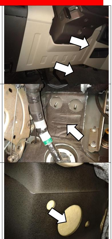
**5.** Install module below the dashboard, securing it with zip ties, connect it to the harness.
