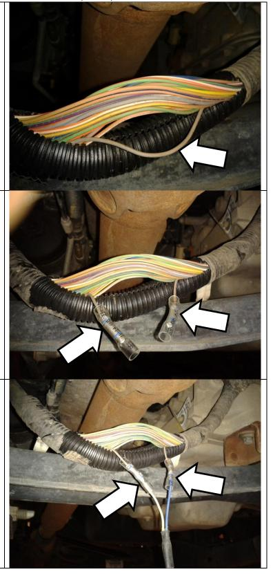
27. Seal the heat shrink connectors using a heat gun or suitable heat source. Put the wires back into the wire loom and wrap the section with electrical tape. Double check that the wiring is well clear of the forward drive shaft (if equipped).
