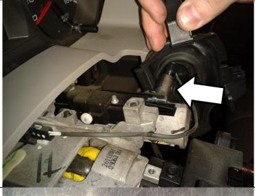
15. Remove and discard the white plastic securing clip from both the old and new shift lever electrical connectors to make boot transfer easier.
