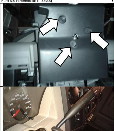
Pop the electrical connector for the shift lever out of the mounting location on the top of the steering column. Disconnect the shift lever wire from the vehicle.
