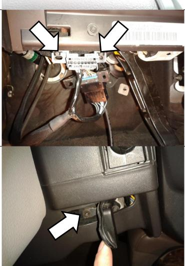
10. Remove the steering column tilt handle rubber grommet and remove handle by removing the T20 screw securing it. 11. Remove the 5.5mm screws securing the bottom of the steering column cover. Separate column covers using trim removal tool or other suitable tool. The two halves snap together and must be pried apart. This may be easier if the shift lever is moved out of Park.
