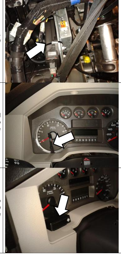
8. NOTE On models without a mileage reset button in the instrument cluster, it is possible to install the display above the shift lever on the right side of the instrument cluster instead of the left. This is left to the customer's preference.
