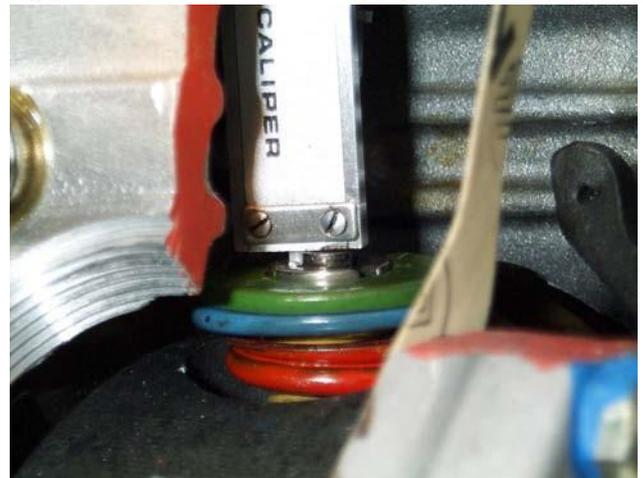
18. Remove adjusting nut using a long thin screwdriver and a pencil magnet.
