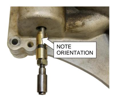
Give the clip a pinch before installing to ensure a strong fit.
