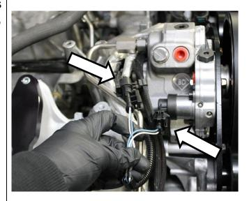
35. Loop supplied harness around toward OEM CP4 pump, and pull underneath coolant crossover passage. Plug harness into OEM CP4 pump.
