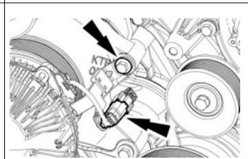
45. Re-install fan stator using three(3) of the OEM fasteners, as shown. Using a 13mm socket, torque to 12.5 ft-lbs (150 in-lbs).
