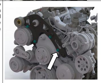
27. Install OEM idler pulleys as shown using OEM hardware. Using a 15mm socket, torque fasteners to 35 ft-lbs.
