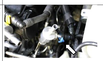
Insert 1500723 quick-disconnect fitting into end of supplied 1/2in fuel hose, and secure with 1452821 gear clamp.
