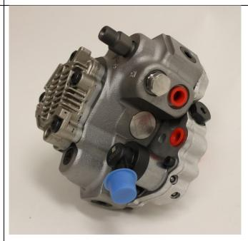
22. Mount CP3 pump to CP3 bracket 1500714. Use three(3) supplied 1453934 Bolts, six(6) 1401556 Washers, and three(3) FT-1190681 Nuts. Torque fasteners to 20 ft-lbs using a 13mm socket, and 13mm wrench.
