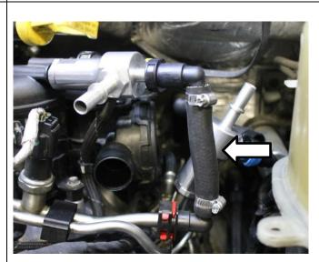
57. Locate OEM fuel return quick-disconnect (seen here with blue latch), and remove.
