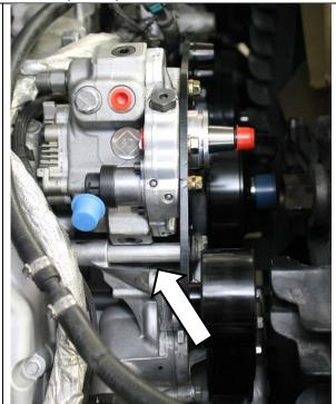
26. Torque all bolts from bracket to engine to 18 ft-lbs, using a 13mm socket. Excluding lower right hand bolt (see arrow). This bolt will be installed with the cooling fan assembly later.
