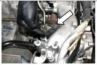
8. Remove the grey plastic insert from the OEM CP4 connector using a small screw driver. This part will be modified to fit the new CP3 to CP4 wiring harness.
