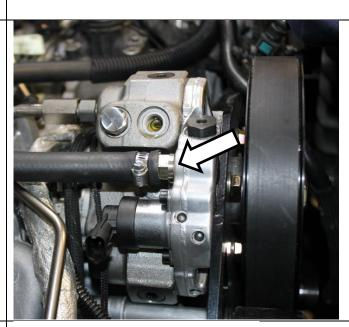
62. Insert 1500727 quick-disconnect fitting into end remaining supplied 1/2in fuel hose, and secure with 1500387 spring clamp.
