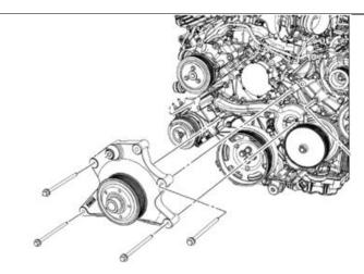
15. Using 13mm Socket, install smooth fan pulley hub CC3Z-8553-C, found in optional kit 1050470-SB. Torque fasteners to 18 ft-lbs.
