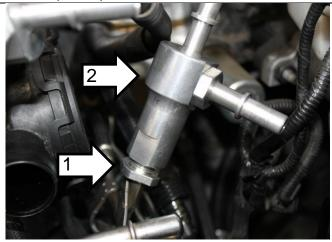
Plug OEM fuel return line onto quickdisconnect adapter as shown, and depress locking collar.
