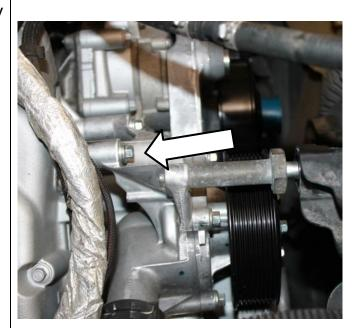
12. Remove both idler pulleys using a 15mm socket. These will be relocated to CP3 bracket, once installed.
