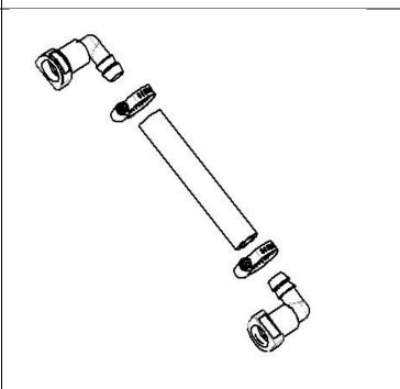
Remove OEM fuel tube assembly, by pinching tabs together on quick-disconnects, and pulling up on colored collars.
