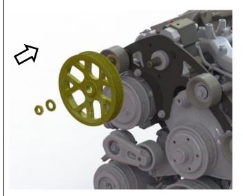
29. Ensure all pulleys are free running and have clearance. If interference exists, it may help to loosen bolts on main bracket and adjust position on engine.
