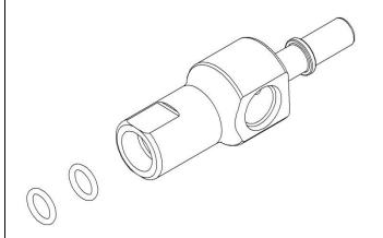
52. Install a 1500721 ORB adapter with O-ring into each 1500719 quick-disconnect adapter as shown. Torque to 15 ft-lbs, using 7/8in wrench.
