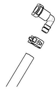
Connect hose to quick-disconnect adapter with OEM return line, and route fuel tube towards CP3 pump return banjo fitting.
