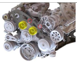
28. Install CP3 drive pulley 1500708 onto pump shaft with washer FT-40388 and jam nut FT-MJ2740000ZP00. Using a 27mm socket, torque nut to 75 ft-lbs.
