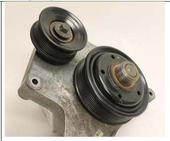
14. Using 13mm socket, remove fan pulley hub from front of engine.
