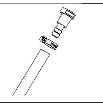
59. Connect hose to quick-disconnect adapter located on fuel filter, and route fuel tube towards CP3 pump feed fitting.
