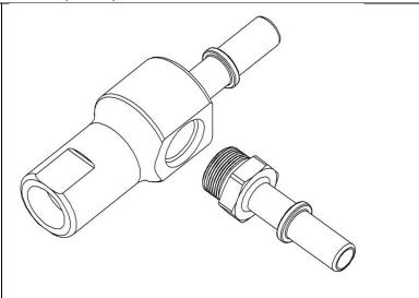
Using 4-1/2 in of supplied ½in hose, use 1452821 gear clamps to secure a 1500727 quick-disconnect fitting in each end as shown.
