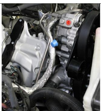
33. Route OEM CP4 pump wiring behind installed CP3 pump as shown.
