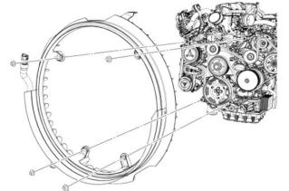
3. Unplug cooling fan connector, and unbolt bracket from engine using a 13mm socket.
