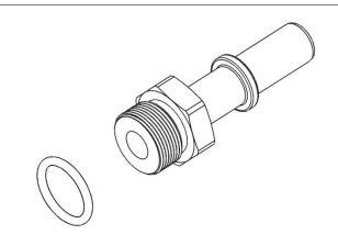
51. Insert two(2) FT-99604842 O-rings into each 1500719 quick-disconnect adapter. They are installed into the internal O-ring grooves inside the large end.
