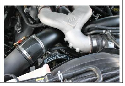
67. Prime fuel system several times using the filter pump, or lift pump and start engine. Check for leaks.
