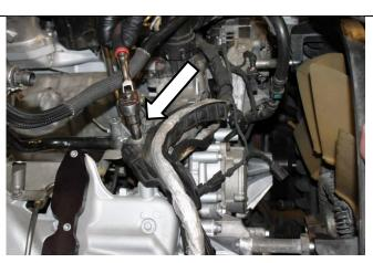
7. Un-plug OEM CP4 pump, and pull wiring out toward front of engine for access to connector.
