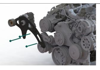
25. Insert stand-off 1500715 between CP3 bracket and engine, using the supplied longer OEM bolt W701629-S437.
