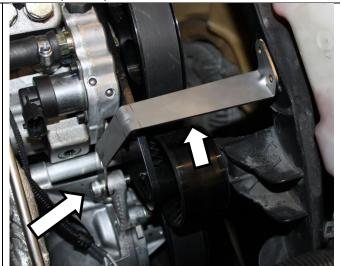
Mark fan stator through holes on 1500725 bracket, and then remove for drilling holes.
