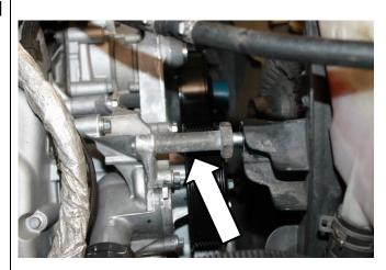
11. Remove upper bolt from secondary water pump, using 10mm socket.
