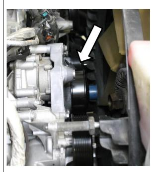
Using 13mm socket, remove three
