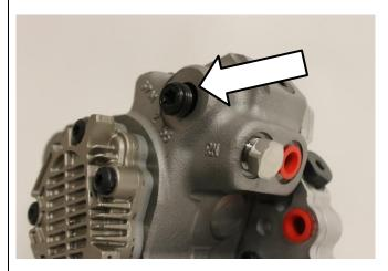
20. Carefully remove spring from OEM plug and install onto new output fitting F00N200499.
