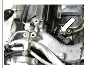
36. Route harness and wiring behind CP3 pump, and ensure wiring is not directly contacting exhaust manifolds, or any other hot surface.
