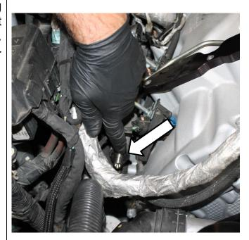
32. Install supplied fuel line 1500716 between the installed fuel rail fitting, and the CP3 output fitting. Torque both ends to 30 ft-lbs using 19mm crows foot wrench.
