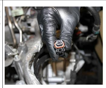
9. Using a small file, remove the keyways (ribs) on both sides of the grey plastic insert. Then install back into OEM CP4 connector.
