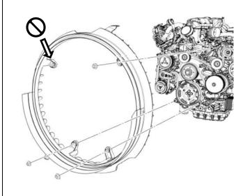
46. Using 1601711 fastener, temporarily install supplied 1500725 stator support bracket onto the passenger side upper stator mount.
