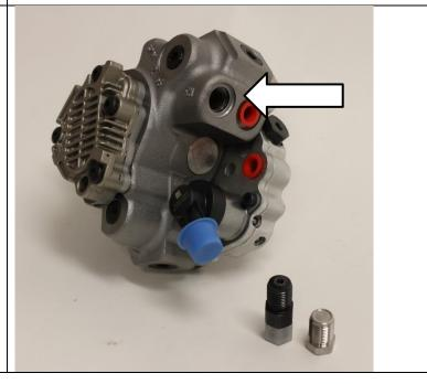
19. Remove OEM plug located adjacent to the output fitting using T50 Torx bit.
