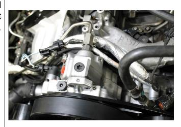
37. Remove the OEM CP3 inlet fitting and transfer the sealing washer over to the new 1502040 HiFlow fitting as shown.
