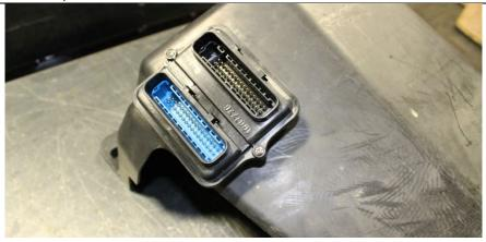
vehicles 23. Connect the with **BLUE** harness the and the BD connector **BLACK** harness with the connector to the BD Tap Shifter control module.
