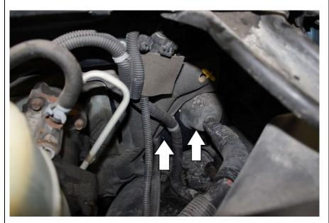
15. Connect the new wiring harness to the shift lever and to the vehicles original shift lever connector. Depending on harness routing in the engine bay, there may be excess wire. Coil wire out of the way of the pedals if necessary.
