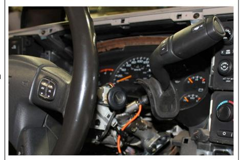
9. Remove the two 10MM bolts securing the transmission control module cover.
