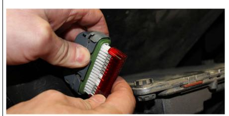
11. Remove the RED retainer on the vehicles transmission harness connector. Install the supplied BLUE retainer. Keep the removed RED key incase the module is ever removed.
