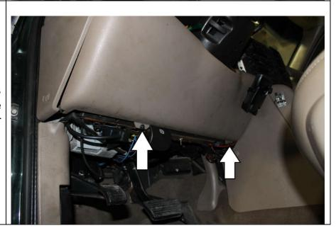
4. Remove the steel plate below the steering column by removing the four 10mm nuts.
