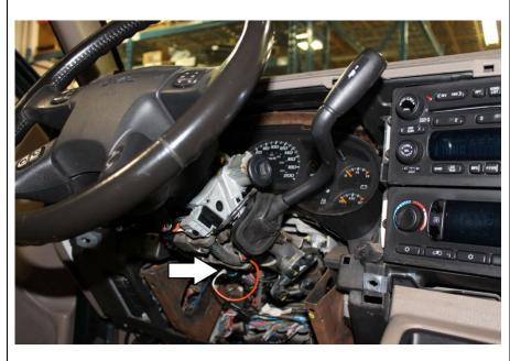
7. Pull back the rubber boot on the shift lever. Using a T27 torx bit, remove the screw attaching the shifter lever to the mechanism in the column.
