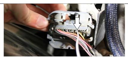
35. Crimp the supplied terminal onto the black wire from the LED. Install into position 20.
