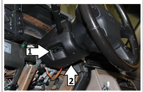
Disconnect the two pin electrical connector running to the original shift lever under the steering column. Remove the two plastic clips holding the shifter wire to the column.
