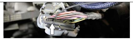
36. Clip the clamshell back together. Reinstall the clear retainer clip. Reattach to TCM.
