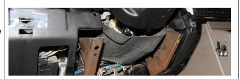
19. Reinstall the trim surrounding the instrument cluster. The interior should now be fully reassembled.
