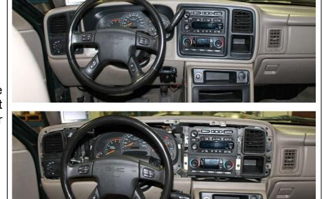
Remove the two 7mm screws from the bottom of the knee bolster and pull bolster outwards.
