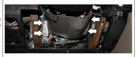
5. Remove the tilt lever from the steering column (1) and the screws from the bottom side (2). Unclip the upper and lower covers. Use care not to break the clips on the covers.
