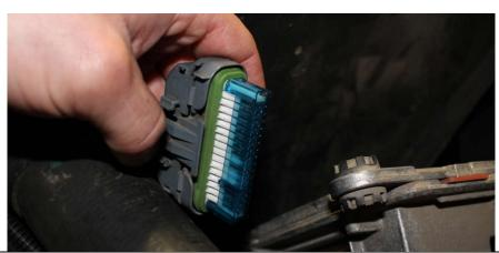
12. Connect the BD Tap Shifter wiring harness RED connector to the vehicles transmission control module.
