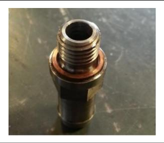
7. Once the washer is switched over, thread the HiFlow fitting into the CP3 inlet. Torque the fitting to 6ft-lb (72in-lb).
