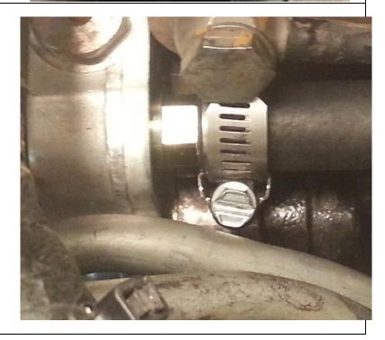
7. If using a BD Flowmax pump. Thread supplied 1/2" barb fitting into the pump inlet and secure with a hose clamp, cut hose to length as necessary.
