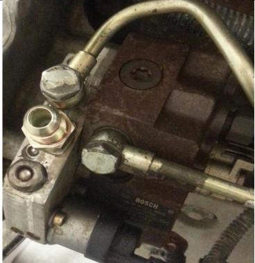
4. Now thread the 8JICF to 90 Hose barb (1502038) onto the JIC fitting and tighten with an open end wrench. Tighten the pair of fittings until the lower M12 fitting just begins to turn and then stop.
