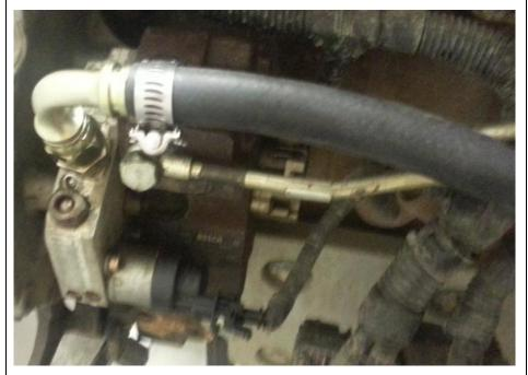
7. If using a BD Flowmax pump. Thread supplied 1/2" barb fitting into the pump inlet and secure with a hose clamp, cut hose to length as necessary.
