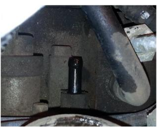
Remove the CP3 inlet fitting and transfer the sealing washer over to the new HiFlow fitting as shown.
