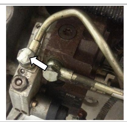
Insert the M12 to -8JIC (1502033) adapter and torque to 6ft-lb (72in-lb).
