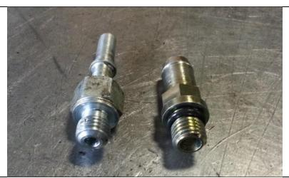
4. Once the O-ring is switched over, thread the HiFlow fitting into the CP3 inlet. **Torque the fitting to 6ft-lb (72in-lb)**.
