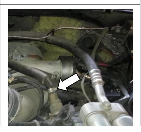
4. Now remove the steel coolant pipe from the top of the motor.
