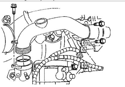
Looking down in the valley, the CP3 inlet fitting should be visible. Remove the hose clamp and pull off the inlet hose.
