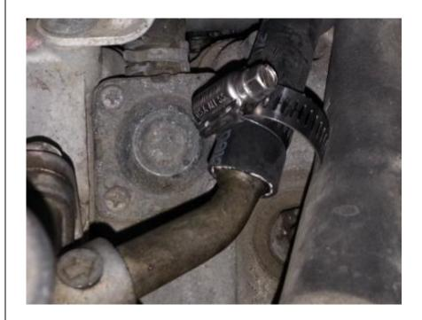
13. Ensure the abrasion sleeve is in the correct position and the hose is secured properly to avoid leaks and chafing.
