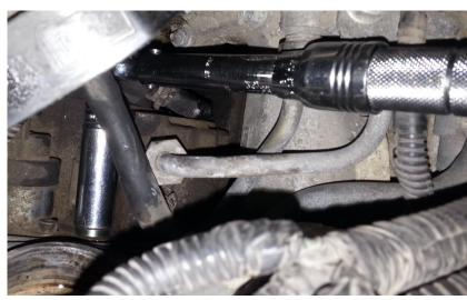
8. Remove the two stock fuel supply lines from the filter head to CP3 inlet. These are the lines with the arrow pointing away from the filter head (circled).
