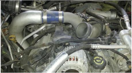
3. Unscrew the band clamp and remove the turbocharger coolant supply line from the hose nipple.
