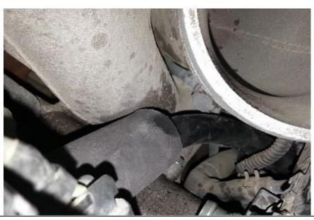
14. Using quick disconnect tool, remove the supply line on the rear driver's side of the engine. The turbo outlet boot may need removal to gain access.
