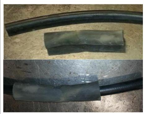
10. Push the 1/2" hose over the HiFlow barb and secure tightly with a socket.
