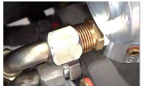
**C.** Attach the assembled fuel line to the FASS and engine.
