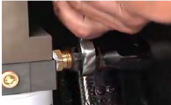
**B.** Attach the fuel supply line from the "E" Port of the FASS System to the injection pump using 10-273, or one of the fittings from the filter housing removed in Step two (2).
