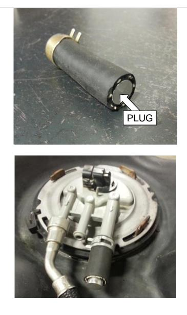
Note: If the sump leaks from the O-Ring, remove the sump and check the cut flange for burrs or cuts in the tank surface.
