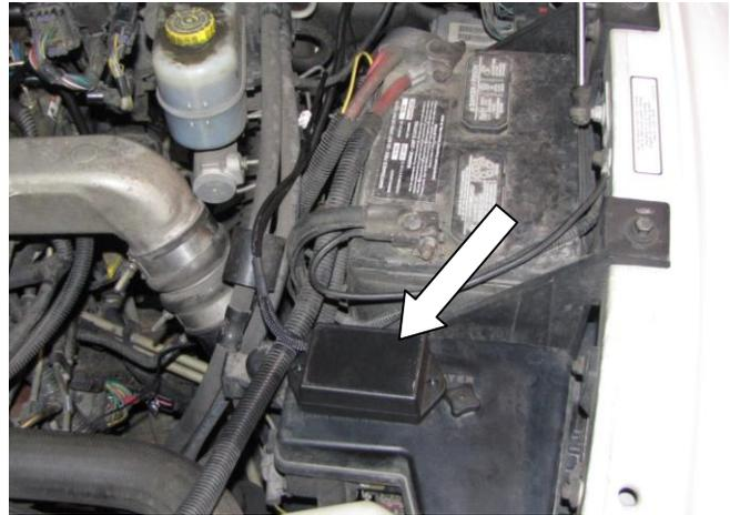
3. Route TTVA plug connectors down the firewall and under the vehicle.
