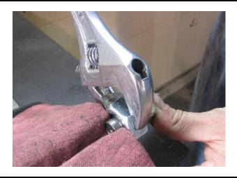
7. Release the valve from the vise and remove the spring to insert the supplied *hardened steel shims* into the valve.
