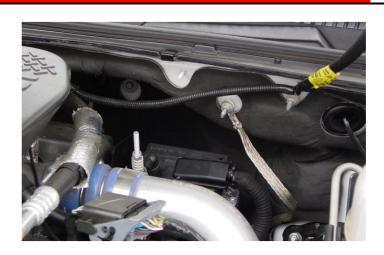
Remove the 5 bolts shown, four on the case and 1 on the metal tubing shown. Remove black metal casing under the bolts to access the fuel pressure valve. (12mm & 10mm Socket)
