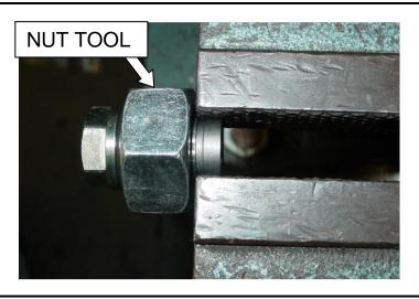
5. Use a 1 3/8" or 30mm wrench to unscrew the nut tool this will remove the **spring loaded** valve cap.
