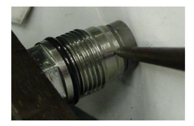
10. Reinstall fuel pressure relief valve back into the fuel rail. (torque to 76 ft/lbs)
