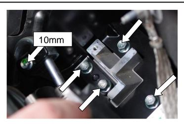
Once the glow plug controller is removed you can access the fuel pressure valve. Unscrew valve to detach from fuel rail. (18mm Wrench or Socket)
