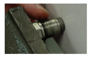
9. Using a punch and small hammer re-strike the factory indentations along the lip where the valve casing covers the valve cap (3 places). You may need to rotate the valve to access the three locations by slightly loosening the vise ensuring the cap stays fully seated in the valve while it is being rotated.
