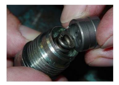
8. Place the valve back into the vise with a piece of cardboard behind the valve cap to prevent damage to the valve seal surface. Tighten the vise until snug so the valve cap re-enters the valve until fully seated.
