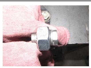
6. Unthread nut tool against vise using a wrench to remove the valve cap.
