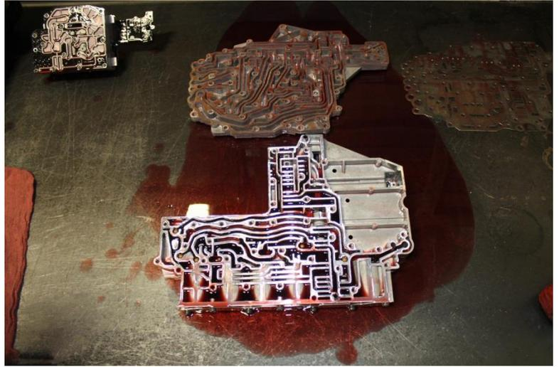
17. Thoroughly clean the bottom (smaller) half of the valve body. Locate the passage to be drilled.
