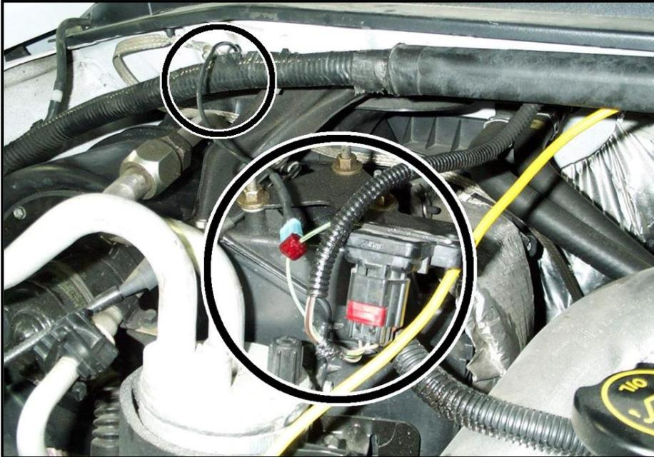
To install the electronic boost cut-off, locate the map sensor located on the passenger side of the engine compartment near the rear. Attach the T-Tap or Posi-Tap to the center wire (Light Green/Black trace) and connect the other end to the chassis ground nearby. This device prevents the SES light (high boost code) from appearing.
