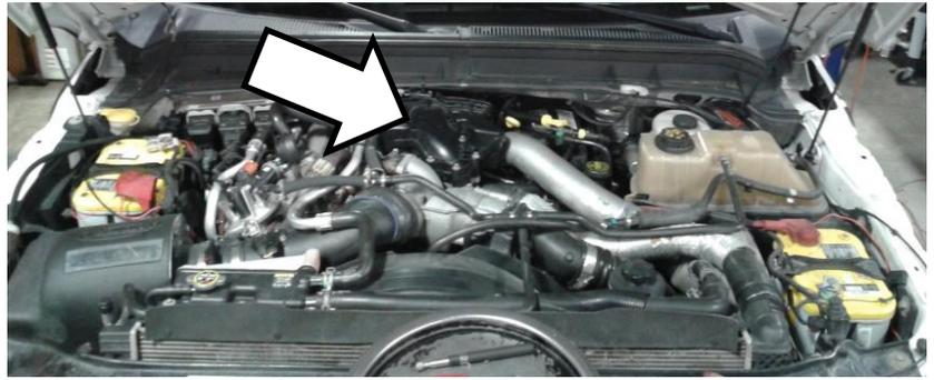
20. Disconnect the wire connection from the MAP sensor on the top of the intake manifold.
