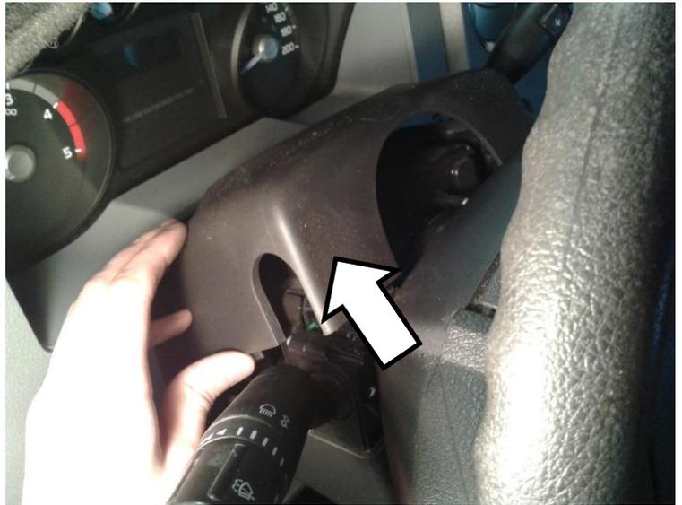
7. Locate the shift lever connector just behind the hazard lamp switch on the top of the steering column.
