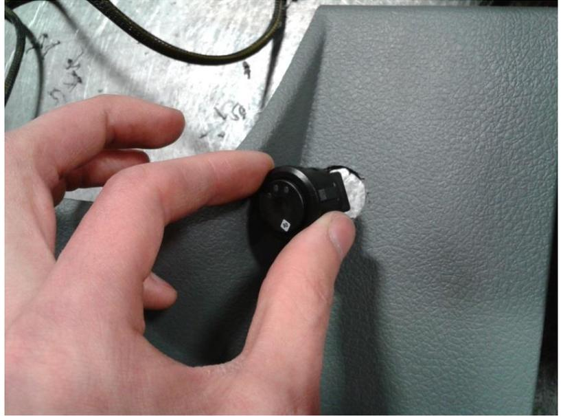
Install supplied switch decal onto the dash aligning the notch on the decal with the notch you created. Then install the switch into the hole.
