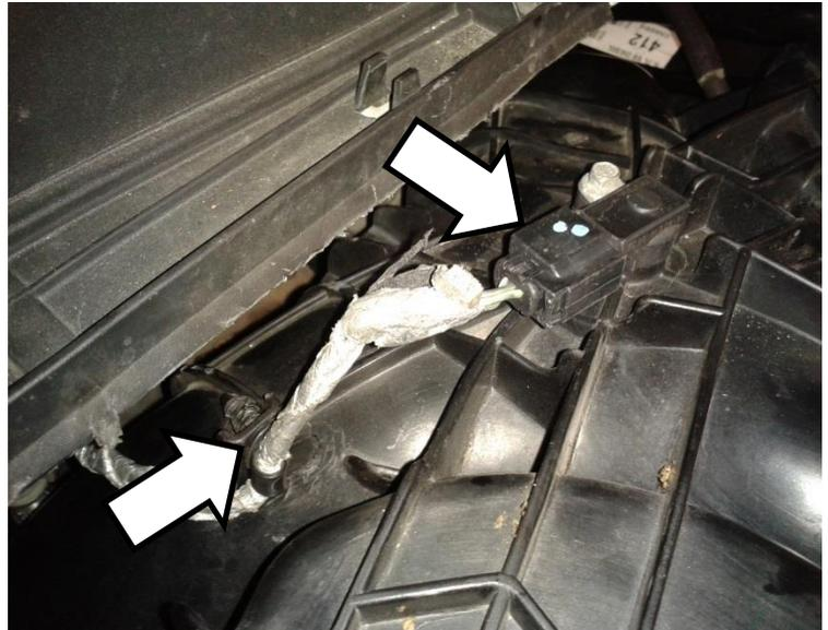
21. Disconnect the coolant tube hold down clip from the intake manifold.
