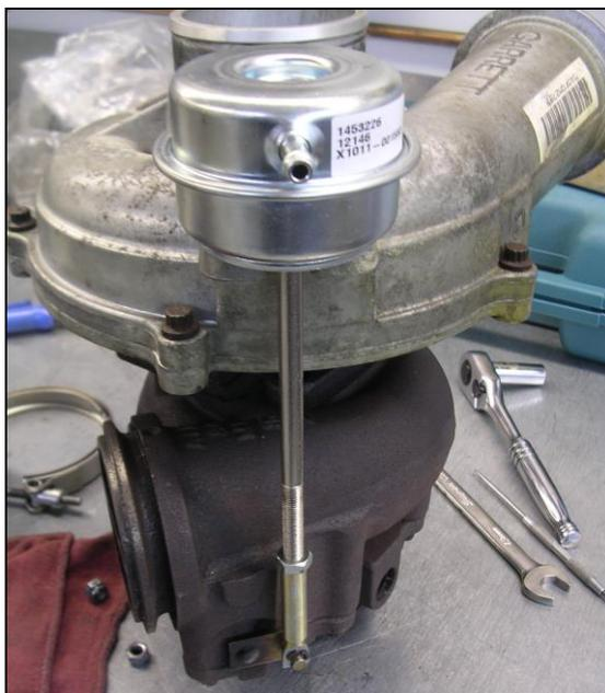
The waste gate is preset to allow 25psi of boost pressure. One full turn of the rod clockwise (shortening the rod) will increase boost pressure by 5psi. One half turn will increase boost pressure by 2.5psi.
