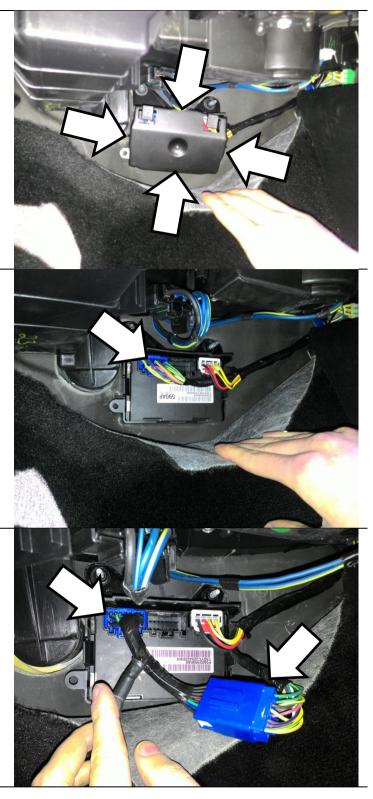
Install the two supplied relays into the BD wiring harness.
