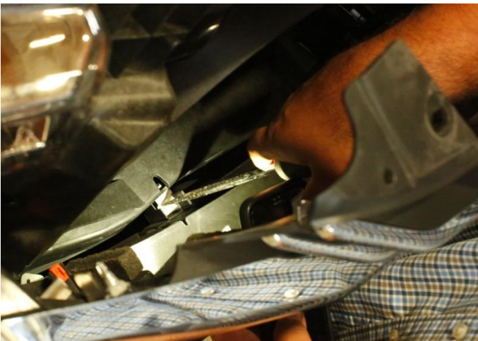
Step 5: Before removing the grill, you have to detach grill from headlight, grip the upper and lower half of grill and tug. Repeat process on right side.
