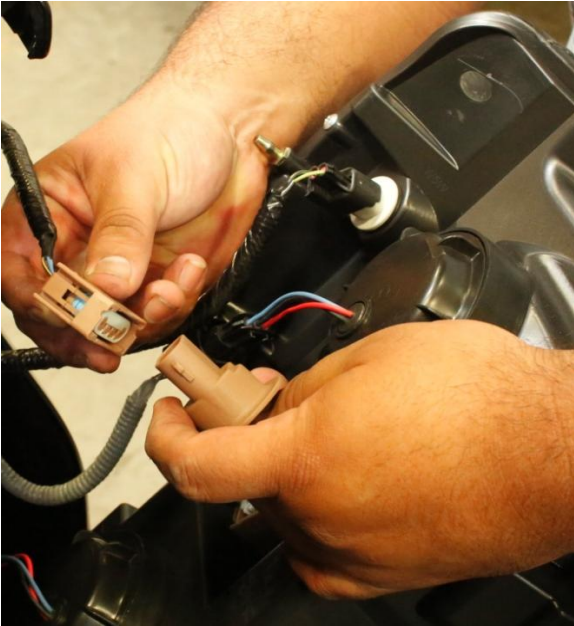
Step 14: Install the Anzo headlight, connect harness to new headlight.
