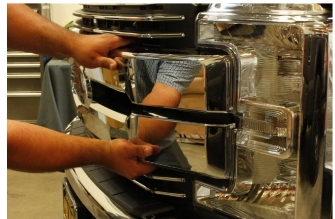
Step 6: Grip the upper and lower half of the grill and tug on the grill until you detach two fasteners from the headlight.
