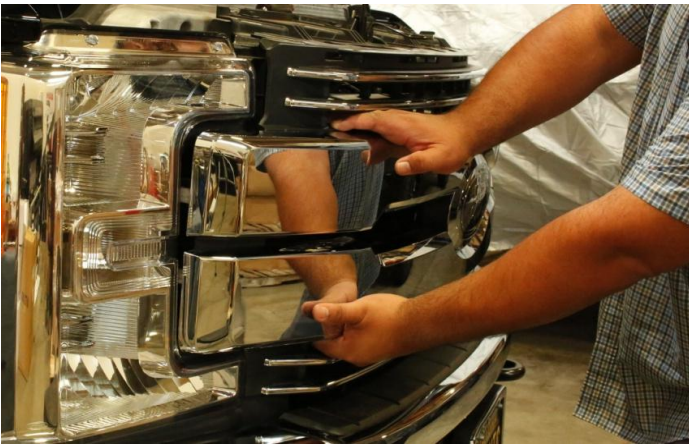
Step 5: Before removing the grill, you have to detach grill from headlight, grip the upper and lower half of grill and tug. Repeat process on right side.
