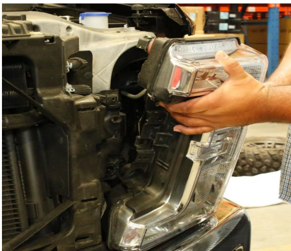
Step 12: Push down on the OEM headlight and pull out from the top.
