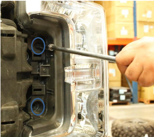
Step 9: In order to remove OEM headlight, you have to remove a total of four 10mm bolts.
