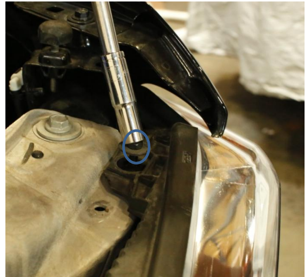
Step 10: Remove one 10mm bolt from top of headlight.
