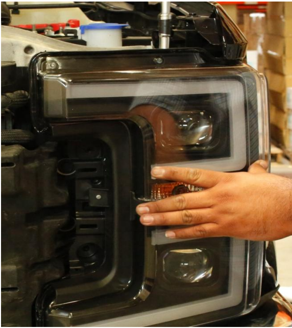
Step 16: Hold the Anzo headlight in place and secure headlight with factory four 10mm bolts.
