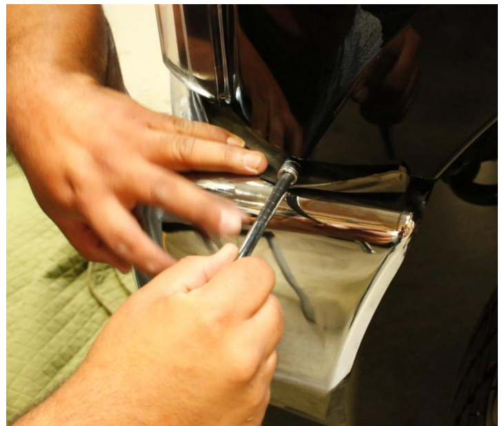
Step 17: Check fitment before tightening down all four 10mm bolts.
