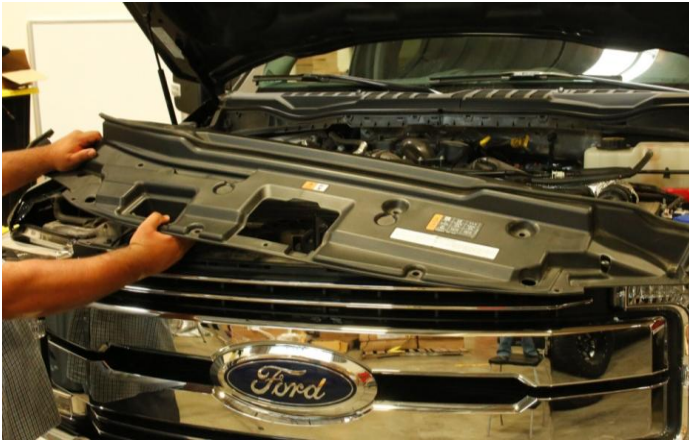
Step 3: Remove radiator shroud and store in safe place.
