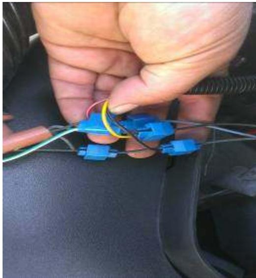
**Step 7-** Once you have the wires all spliced in you can test them to make sure they are working properly by turning on your running lights then your turn signal and then hazards. Once you have tested all the functions you can put your light back in the vehicle and proceed to the other side.
