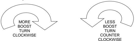
To increase the boost pressure, you will have sufficient energy to drive the turbo faster. Once you have turned the rod to the desired position, re-install the circlip and lock the jam nut.
