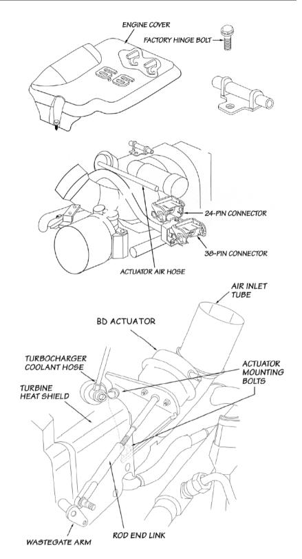
Using the two 12mm bolts, mount the BD actuator in place of the factory wastegate. Securely tighten the two bolts.
