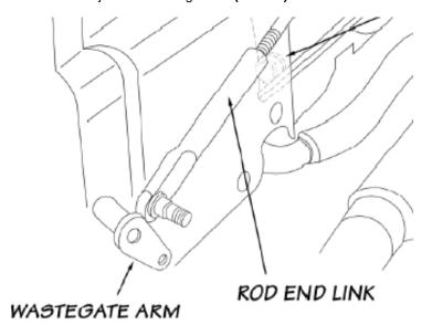
Install the supplied wastegate hose on the actuator nipple and on the factory compressor housing nipple. Secure the connection with the crimp style clamps.
