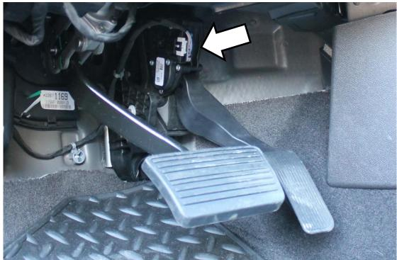
3. Connect supplied wiring harness to the sensor and connect the other end to the factory wiring harness. Secure harness with zip ties so that it does not interfere with pedal operation. Removal of the knee bolster may ease installation.
