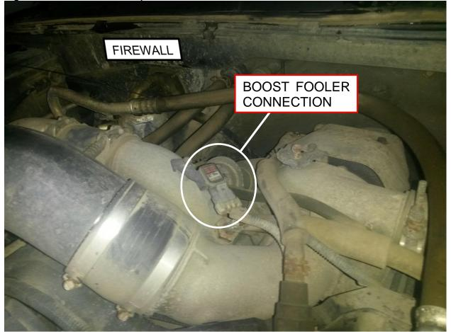
Unplug the factory harness from the boost pressure sensor. Plug the BD Boost Fooler inline with the MAP sensor and the factory harness.
