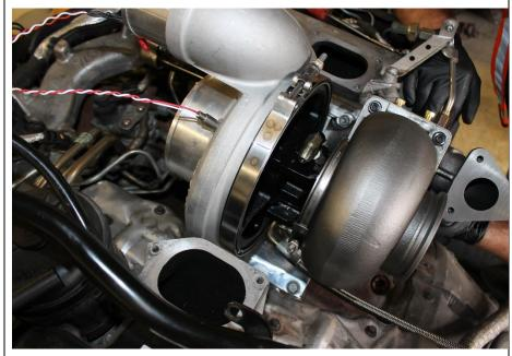
**3.16** Install the oil feed line, take care to assure this line is clear of the driver side manifold, turbine housing and other sources of heat or any edges on which this line could wear on. When tightened in final position the oil feed line should be free from rubbing all other items by 1/2 Inch.
