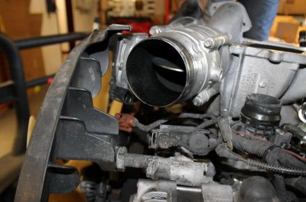
**R2.7** Using an 8mm socket, loosen the front and rear intake boots to the turbo, these boots can be detached when the turbo has been removed.
