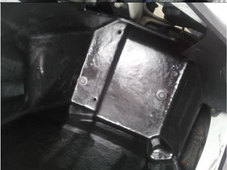
**10.9** Reinstall the radiator screw and air box bracket as shown.
