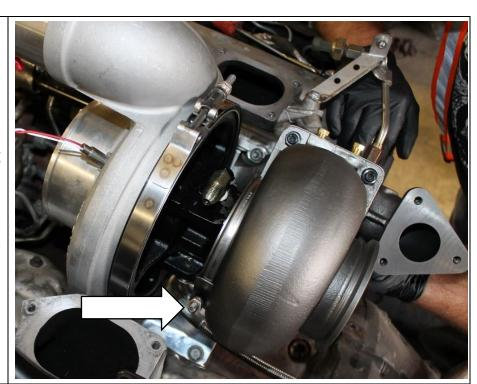
**3.13** Install the 2 oil drains bolts (1302108) using a 13mm socket and torque to 32 ft.lbs securing it to the CHRA.
