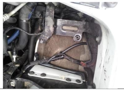
**10.7** Remove the OEM rubber air box mounts and install the 2 1456737 M8 U nuts as shown onto the air box mount.
