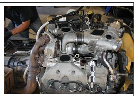
**R2.8** Using a 10mm socket remove the 3 bolts holding the lower cast aluminum intake. The lower intake can then be removed.
