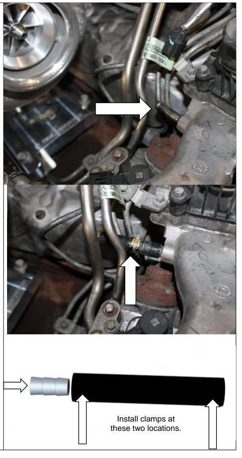
**3.17** Install the turbocharger coolant port block off plug (1462122) in the OE tube located near the CP4. Use the supplied spring clamps (CTL-11), along with the section of 3/8" diameter X 3" L hose provided. This completes this section of the install.
