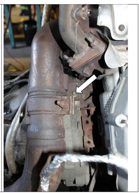
R3.3 Using an 11mm Socket, loosen the V band clamp from the turbocharger turbine housing outlet to the stock downpipe. At this point the downpipe can be removed.
