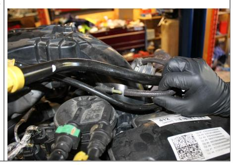
**R2.4** Using an 8mm, socket remove the 15 upper intake bolts. The upper intake can now be removed.
