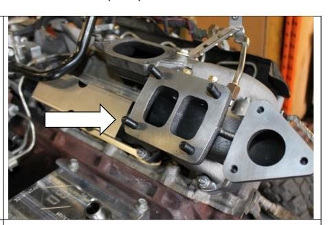
**2.9** Reinstall the coolant tube at this time using a 8mm socket.
