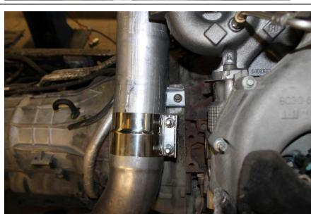
**6.4** Re-use previously removed fastener hardware to secure exhaust ball joint. Ensure female and male ends are clean.
