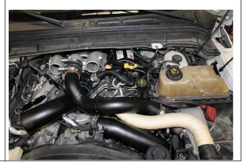
**9.13** Place 2 3" Boots 1405305 onto the intake horns and slide the 1401563 3.5" boot onto the Y pipe end. Install the Y pipe into position as shown. All clamps can be tightened down until spring bound.
