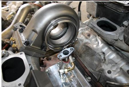
**3.11** Place the turbine housing V band clamp onto the turbine housing past the mounting flange.
