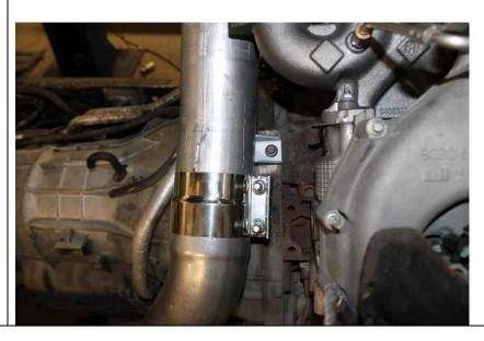
**6.2** Slide the laser cut Lower downpipe flange 1403017-2 onto the lower downpipe 1403017-1.
