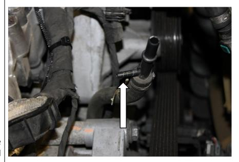
**7.8** Cap the shown location where the wastegate actuator solenoid was fed using the supplied Rubber bullet cap (1900068)
