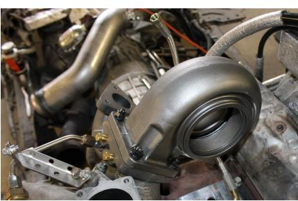
**3.5** Install the 1453144 90° oil feed fitting in the orientation shown. Use pipe sealant or teflon tape. Do not use excessive amounts of sealant, as this could cause oil contamination.
