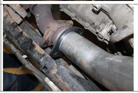
**6.5** Align the 4" lap exhaust clamp as shown and tighten to 45-60 ft. lbs.
