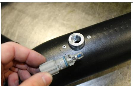
**9.3** Insert the breather crank case adapter 1403043-2 into the 1403043-1 boot as shown and secure with a 32mm clamp (1302197).
