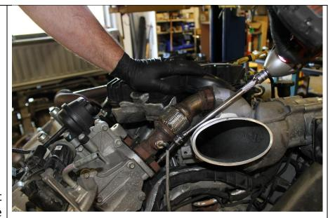
**R1.4** Unplug the EGR outlet temperature sensor from the harness and using an 8mm socket remove the lower EGR outlet tube.
