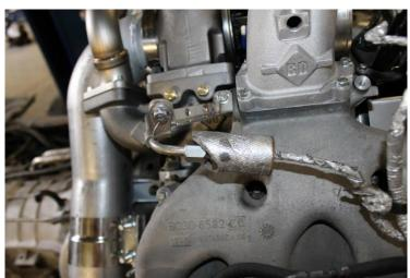
**7.2** Install the MAP sensor onto the passenger side intake horn, use the provided M6x18mm 1505022 bolt and torque to 89 in. lbs.
