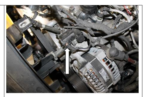
**7.7** Remove the wastegate actuator solenoid and the vacuum tubing lines routed both toward the driver side and passenger Side at this time. Remove the 2 bolts with an 8mm socket. The harness and plugs related to these items can be zip tied and taped up / sealed if wished.
