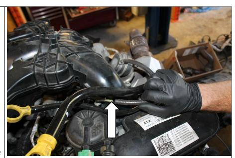
**R2.3** Disconnect the turbochargers wastegate actuator tube on the intake side as shown.
