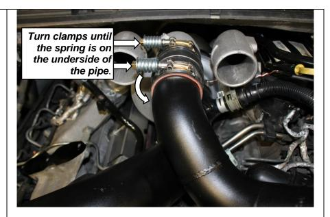
**9.12** Install the 3" Hot side CAC Tube 1403031 with 2 3" Boots 1405305 and 2 3" clamps 1405211. Place the T Bolts on the bottom side and pointing towards the passenger side. All clamps can be tightened down until spring bound.
