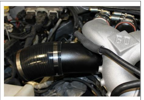
10.12 Place the 2924 air filter into the air box before installing the 1403041 rotary molded intake tube. Slide the tube on an offset just behind the 22° boot. Seat the tube into the air filter as you slide it into place. The 22° boot outlet end can then be seated. Align the tube and boot into position and tighten all clamps.
