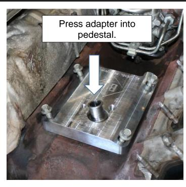
**1.2** Place a new OEM Ford turbocharger pedestal gasket BC3Z-6587-A in place. Place the BD billet aluminum block off pedestal into place and assure it seats correctly on the dowel pins.
