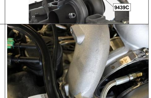
4.2 Install the driver's side intake into place first using the 4 M6 bolts 1900056 and a 10mm socket.
