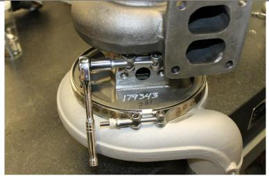
**3.1** Place the turbocharger on a bench with the compressor cover side down and carefully remove the Turbine Housing from the turbocharger super core / CHRA. Assure not to hit the turbine blades causing any damage.
