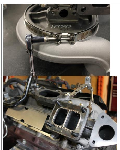
**3.3** Place the 2475042 T4 gasket onto the manifold.
