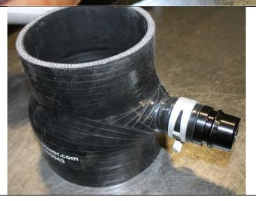
**9.4** Install the assembled 1403043-1 intake boot onto the Turbocharger at the shown angle. We recommend placing the 1405237 Gear Clamp in the shown orientation.
