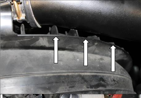
**9.9** Install the 3.5" lower CAC tube as shown. Assure the 3" intercooler joint snaps into place. Do not tighten the clamps until aligned (see photo). The tube should be aligned compared to the fan shroud. The end of the tube should sit almost flush with the tab when lifted forward. All clamps can be tightened until spring is bound.
