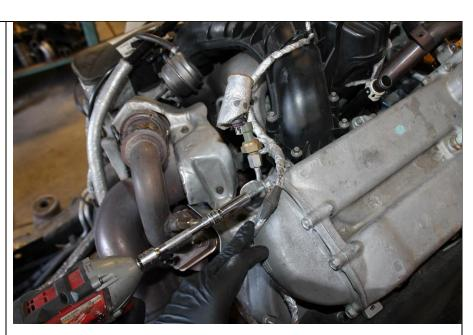
**R1.3** Using an 8mm socket remove the exhaust manifold to EGR upper exhaust tube from the cooler.
