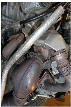
**R3.4** Using an 11mm socket remove the V band clamps from the exhaust manifolds to the up pipe tubes, they can be slid down into the shown position sitting on the tubes, they do not need to be fully removed.
