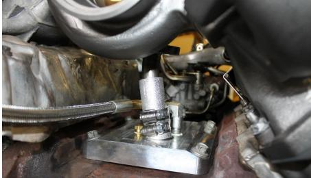
**3.10** The 148062 oil drain gasket can be placed in position now for when the CHRA is installed, or it can be slid into position after the CHRA is installed.
