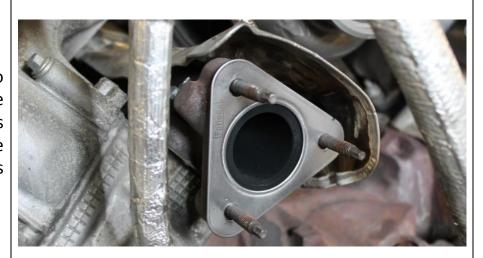
**5.2** During this section assure the transmission dipstick is on the inside or front of the cross over tube. It will need to be massaged into shape to clear in the following step.
