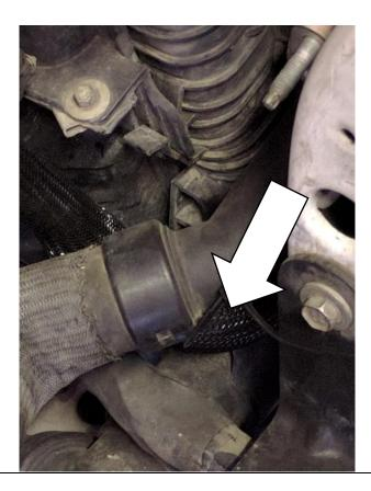
10.3 On the 1403040 BD air box, drill the 2 indented marks shown through with a 1/4" drill bit.
