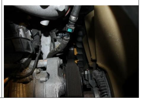
**9.15** Cut the passenger side stock T Junction out on the 5/16" coolant line.
