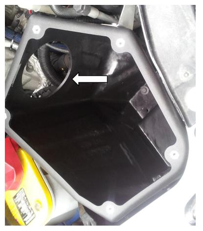
**10.11** Install the 1403043-3 22° boot onto the steel 4" tube with 2x 1453701 clamps slide the clamps into place to be tightened later.
