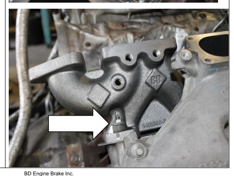
**2.5** Install the (EBP) exhaust back pressure JIC fitting into the manifold (5/16" X -8 JICM).
