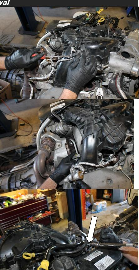
**R2.2** Using an 8mm socket remove the two bolts holding the two dipsticks to the intake on the driver's side.
