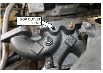
**2.8** Install the M10x25mm 1462431 flange studs into the manifolds T4 Flange. The shorter thread ends goes into the manifold.
