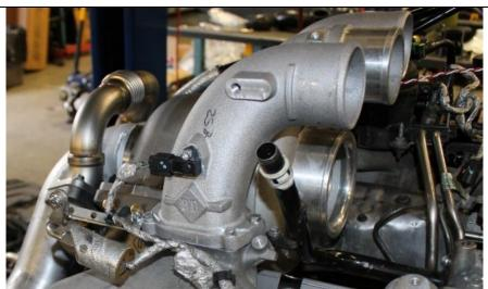
**7.4** Place the lower coolant block off plate 1900082 against the factory EGR Cooler surface.
