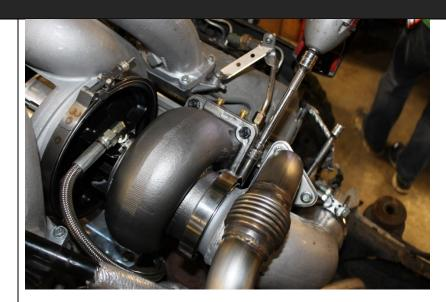
6.1 At the rear of the turbine housing slide the 1453602 downpipe clamp onto the turbine outlet past the flange and place the upper downpipe 1403016 into position, partially install the OE mounting bolt and align the downpipe to the flange. Tighten the V Band clamp followed by the OE mounting bolt and torque the mounting bolt to 22 ft. lbs.
