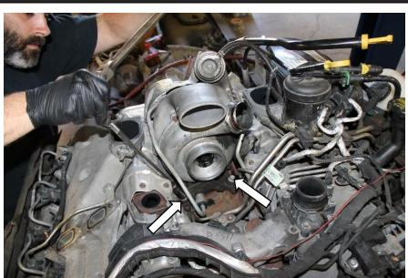
**R4.2** Remove the turbocharger coolant return line found on the driver's side, this simplified by removing the spring clamp on the front of the tube near the coolant cross over in front of the charger. You may also remove the E Clip to allow this tube to be released, this is not required.
