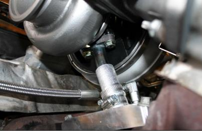
**3.14** Tighten the oil drain hose gear clamps at this time.
