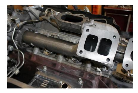
**2.2** Place the T4 flange 1403000 BD manifold into place on the passenger side head. Install the OEM Ford spacers onto the studs after the manifold has been positioned.
