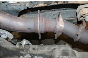
**R3.2** Using a 10mm Socket, remove the bolt holding the OEM cobra downpipe, this is found at between the rear of the engine and the upper down pipe.
