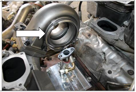
**3.12** Slide the oil drain gasket in place if it is not already. Assure the turbocharger is sitting horizontal and flush with the oil drain flange. Tighten the V band clamp to secure the CHRA to the turbine housing to 90 in.lbs, we recommend the position shown for the V Band bolt.
