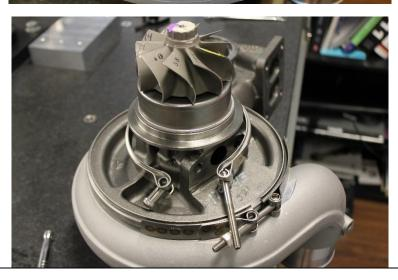
**3.2** The compressor cover V band clamp can be slightly loosened to allow it to be clocked into position once installed. Only loosen until the compressor cover can be rotated with some force and is still held in position.
