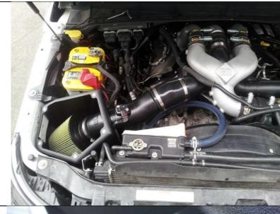
**10.14** Install the OEM MAF sensor into the intake tube as shown, use the provided 2 x 8-32 FT-0173590 and 1403041-1 gasket.
