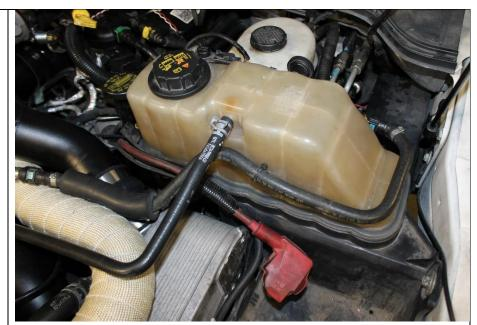
**9.14** Re-install the vacuum and coolant overflow lines into place on the driver's side and the heater line attachment.
