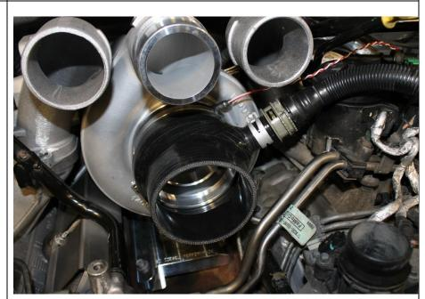
**9.6** Place the 4" Intake Tube Into position as shown, with 1453701 gear clamp installed on the 4-5" intake boot. Do not tighten the 1405237 gear clamp at this time.
