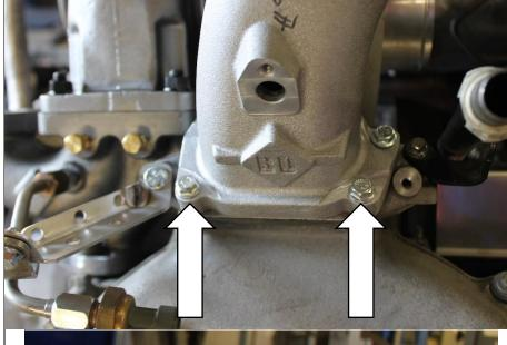
4.4 The 1/8" NPT plugs 1200208 can be installed in each of the intake horns, unless you plan on using aftermarket boost gauges or another injection system or boost pressure accessory.
