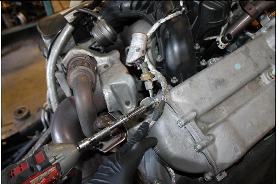
**R1.3** Using an 8mm socket remove the exhaust manifold to EGR upper exhaust tube from the cooler.
