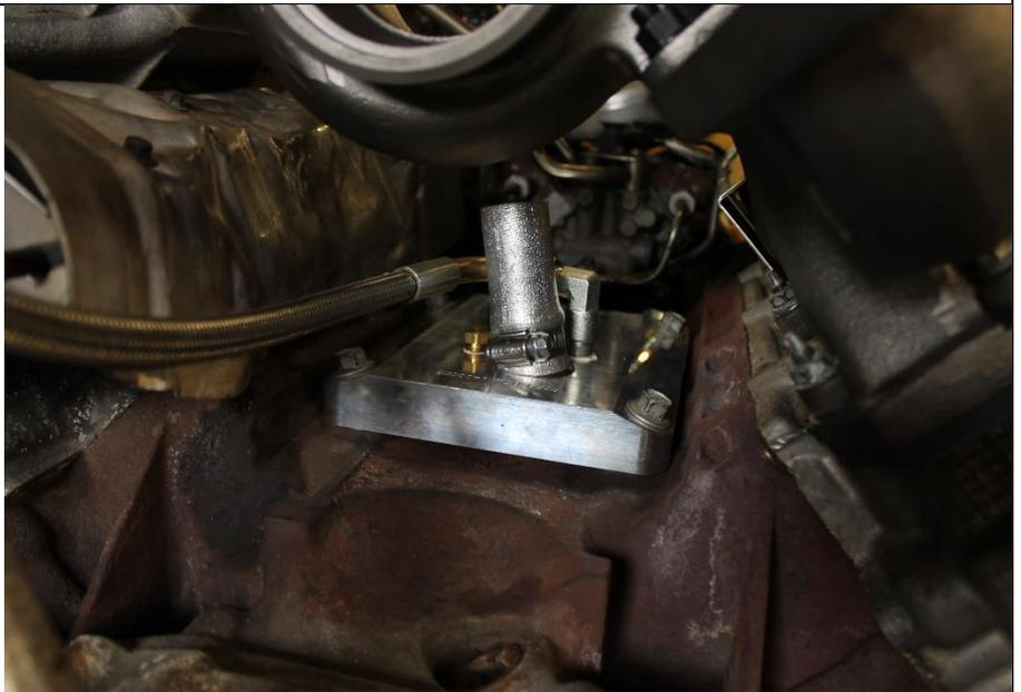
**3.8** Place a second 1453113 gear clamp onto the drain tube hose loose as shown.
