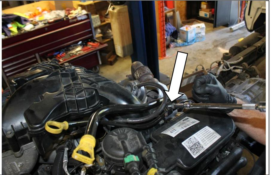
**R2.3** Disconnect the turbochargers wastegate actuator tube on the intake side as shown.
