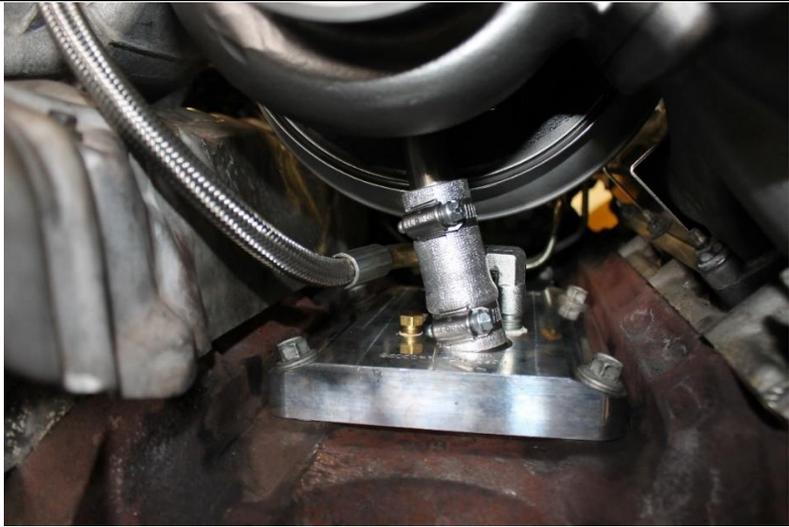
**3.15** Use a small amount of pipe sealant or teflon tape on the threads and install the Oil Feed 90° fitting 1462321 into the CHRA Oil inlet. Do not use excessive amounts of sealant, as this could cause oil contamination.
