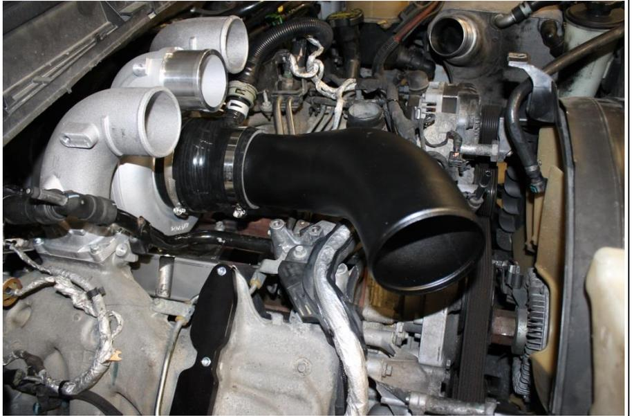
**9.7** Install the only 1407030 clamp provided in the kit for the intercooler and 3.5" clamps as shown on to the 3.5" CAC Tube. Adjust so they are held from rotating but are movable.
