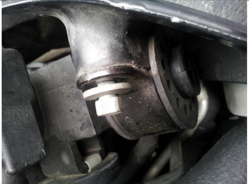
**10.6** If equipped remove the second alternator hook up plug seen on the front of the battery tray and secure out of the way of the new air box attached to the harness below.
