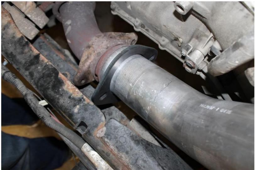
**6.3** With the flange sitting on the tube, install the lower downpipe into position along with the intermediate 4" lap exhaust clamp 1100740.
