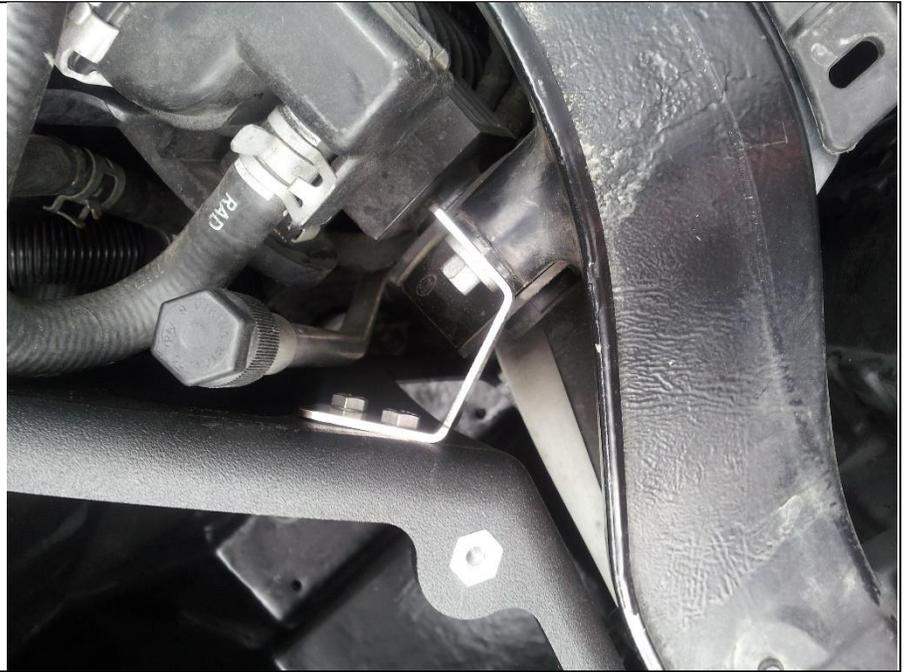
**10.10** Install the 1453820 seal onto the air box outlet hole if it has not been installed already.
