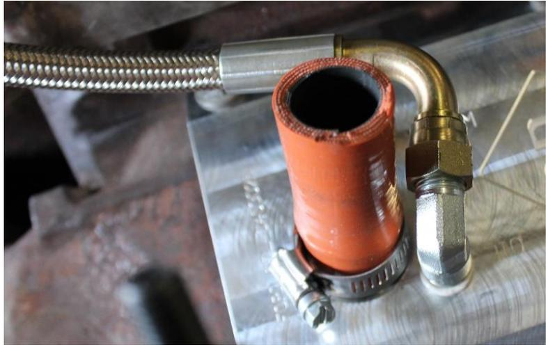
**3.7** Tighten the 1453113 gear clamp to secure oil drain hose.
