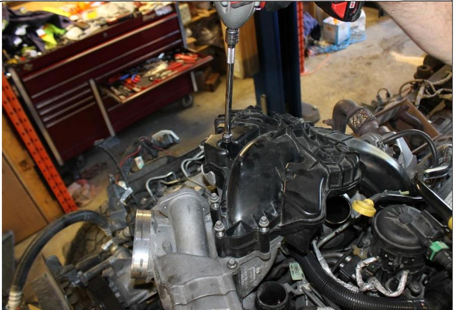
**R2.5** Detach the crank case vent tube from the lower intake / aluminum intake casting to the turbo, this joint is twisted to release. Unplug the sensor cable if you wish to remove this tube until reinstall later.
