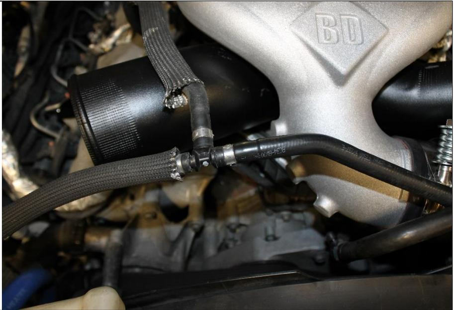
**9.16** Install 1900067 5/16" barb using the supplied CTL-8.5 as shown.
