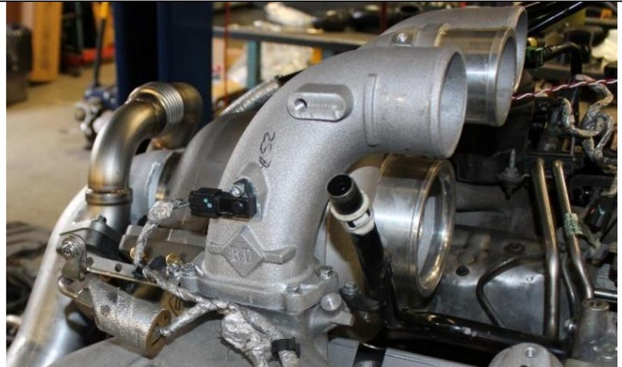
**7.4** Place the lower coolant block off plate 1900082 against the factory EGR Cooler surface.
