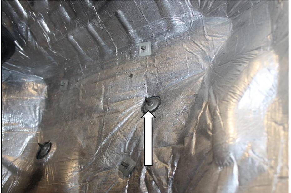
**8.2** At this time the OE Coolant line for the heater can be installed near the Passenger Side intake horn with stock clamps.
