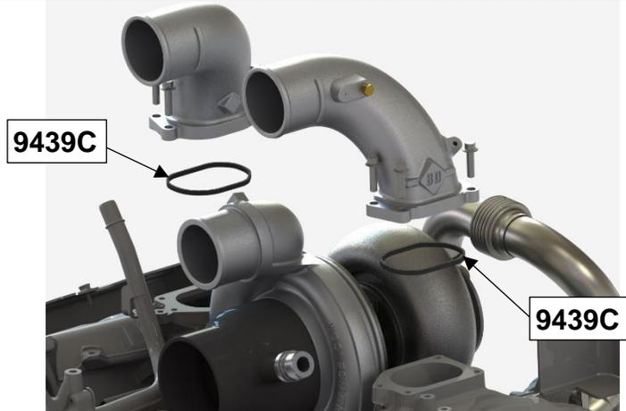
4.2 Install the driver's side intake into place first using the 4 M6 bolts 1900056 and a 10mm socket.
