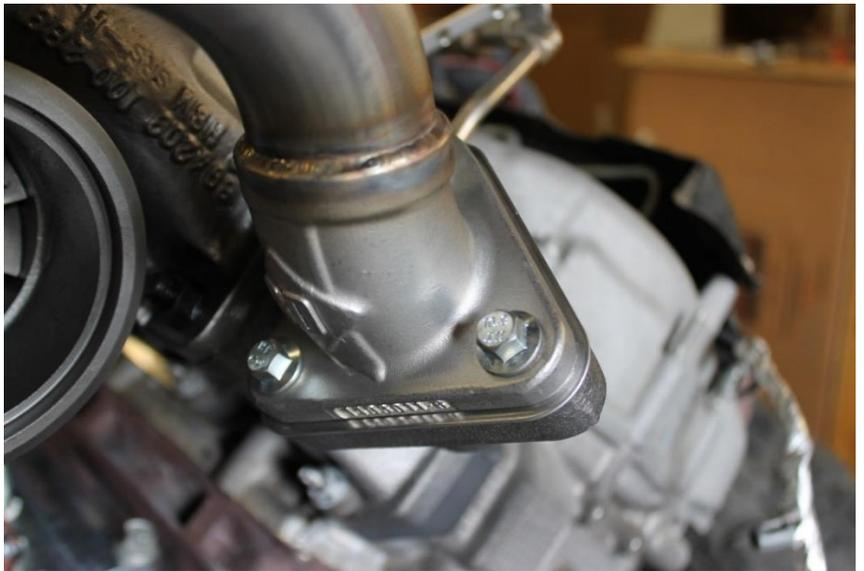
**5.3** Torque the cross over tube bolts and nuts to 18 ft. lbs.
