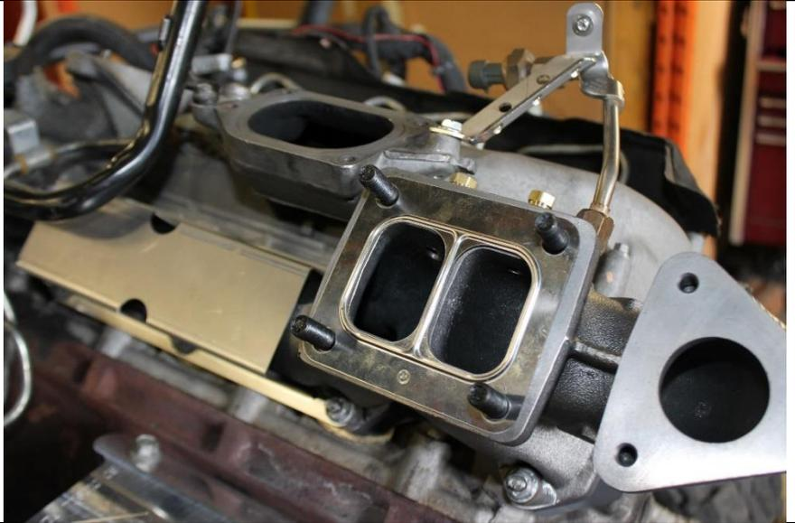
**3.4** Install the turbine housing using 4x 1462441 nuts. Tighten the M10 nuts with a 14mm socket/wrench. Torque to 32 ftlbs in a cross pattern.
