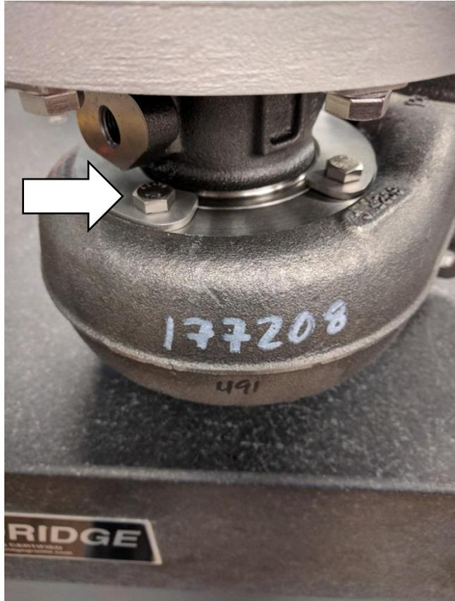
**3.2** The compressor cover bolts can be slightly loosened to allow it to be clocked into position once installed. Only loosen until the compressor cover can be rotated with some force and is still held in position.
