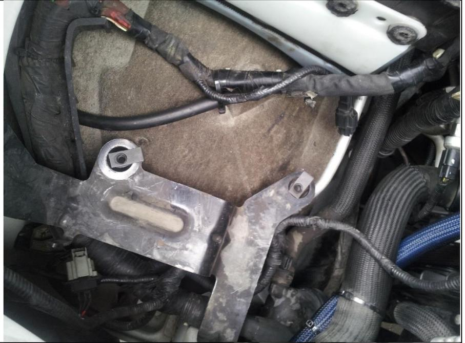
**10.8** Place the air box in position and install the 1456738 M8 bolts.
