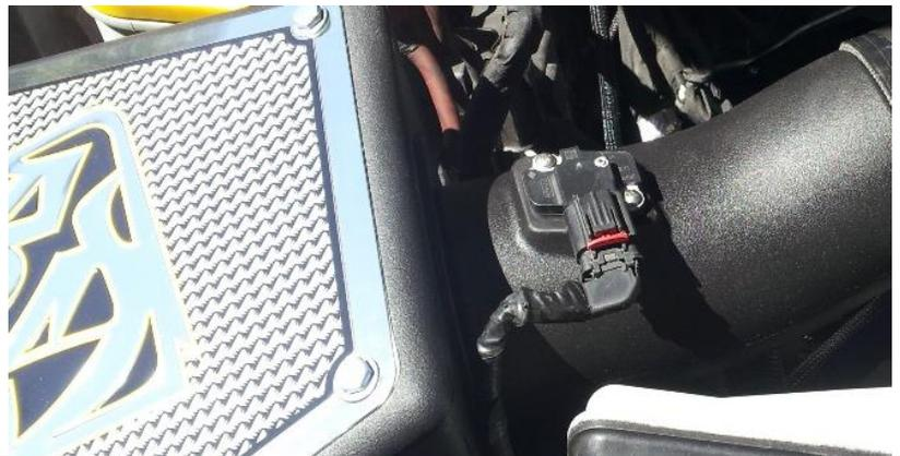
**10.14** Install the air box lid with the 1405422 M6 Stainless Screws. This Completes the intake section install.
