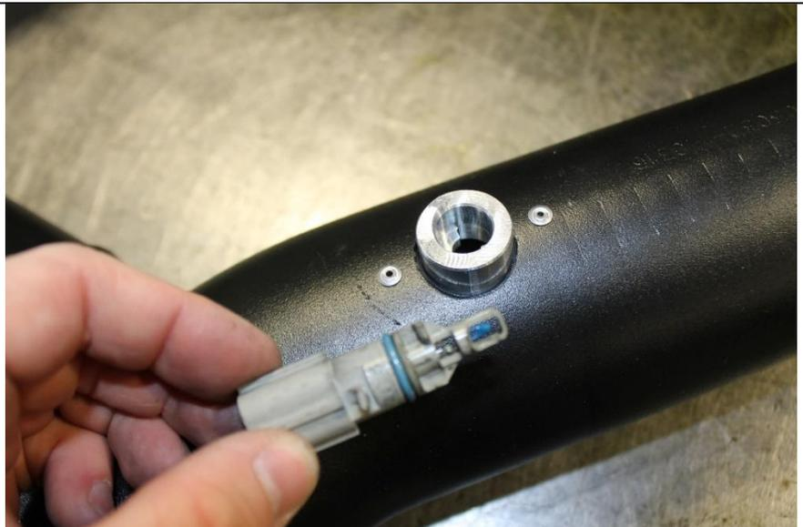
**9.3** Insert the breather crank case adapter 1403043-2 into the 1403036 boot as shown and secure with a 32mm clamp (1302197).
