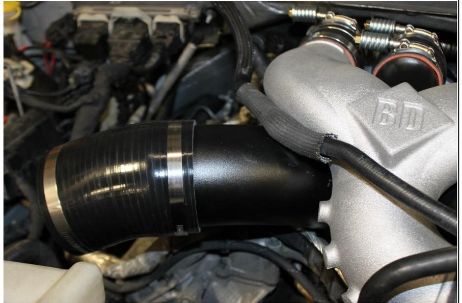
**10.12** Place the 2924 air filter into the air box before installing the 1403041 rotary molded intake tube. Slide the tube on an offset just behind the 22° boot. Seat the tube into the air filter as you slide it into place. The 22° boot outlet end can then be seated. Align the tube and boot into position and tighten all clamps.
