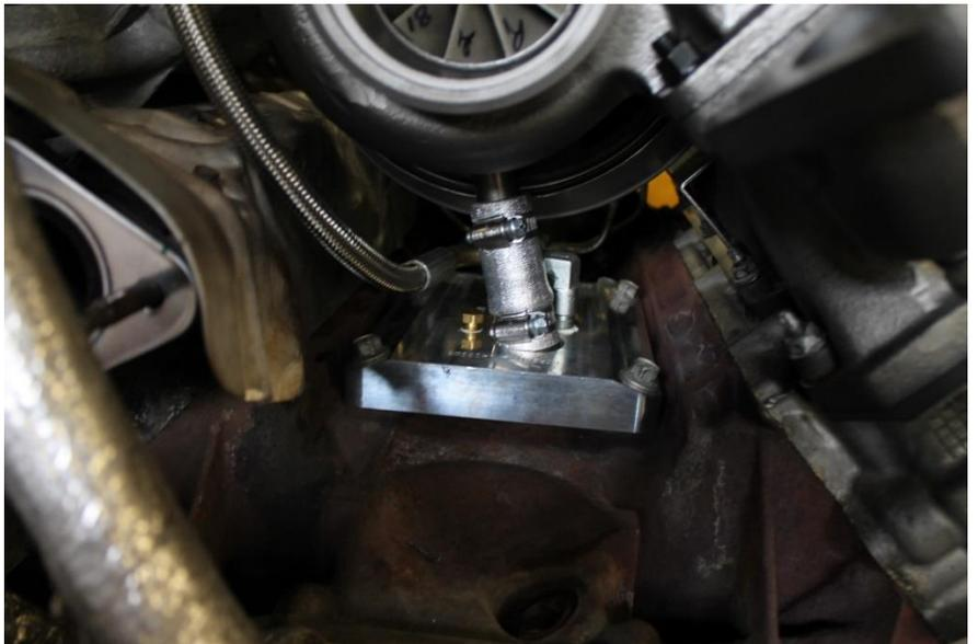
**3.17** Install the turbocharger coolant port block off plug (1462122) in the OE tube located near the CP4. Use the supplied spring clamps (CTL-11), along with the section of 3/8" diameter X 3" L hose provided. This completes this section of the install.
