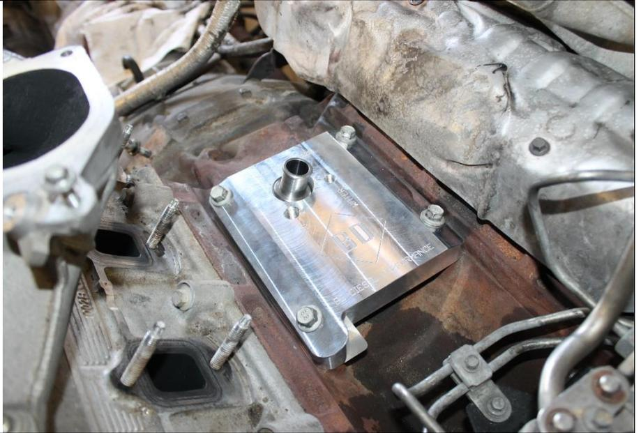
**1.4** Install a 1/8" NPT plug in the water feed location unless you are installing an aftermarket water-cooled wastegate or non-standard watercooler CHRA turbocharger. Use a thread sealant such as Permatex or teflon tape. Insure the NPT is well seated.
