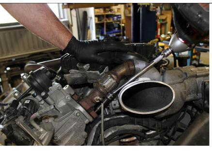
**R1.4** Unplug the EGR outlet temperature sensor from the harness and using an 8mm socket remove the lower EGR outlet tube.
