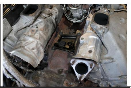
5.0 Passenger Side Manifold Removal
