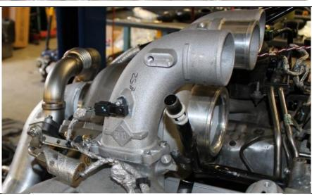
**7.4** Place the lower coolant block off plate 1900082 against the factory EGR Cooler surface.
