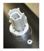
**9.3** Insert the breather crank case adapter 1403043-2 into the 1403036 boot as shown and secure with a 32mm clamp (1302197).
