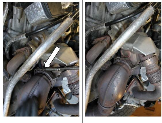
**R3.4** Using an 11mm socket remove the V band clamps from the exhaust manifolds to the up pipe tubes, they can be slid down into the shown position sitting on the tubes, they do not need to be fully removed.
