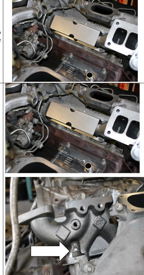
**2.3** Place the 1403002 BD heatshield into place on top of the front of the BD manifold.
