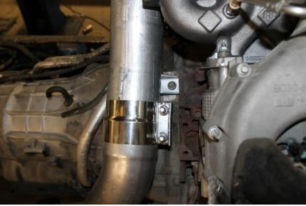
**6.4** Re-use previously removed fastener hardware to secure exhaust ball joint. Ensure female and male ends are clean.
