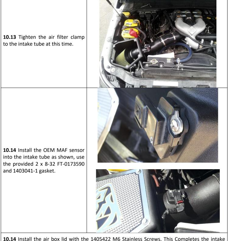
**10.14** Install the air box lid with the 1405422 M6 Stainless Screws. This Completes the intake section install.
