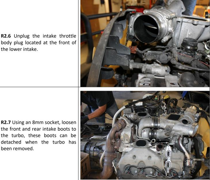
R2.7 Using an 8mm socket, loosen the front and rear intake boots to the turbo, these boots can be detached when the turbo has been removed.
