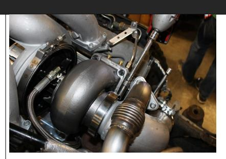
**6.1** At the rear of the turbine housing slide the 1453602 downpipe clamp onto the turbine outlet past the flange and place the upper downpipe 1403016 into position, partially install the OE mounting bolt and align the downpipe to the flange. Tighten the V Band clamp followed by the OE mounting bolt and torque the mounting bolt to 22 ft. lbs.
