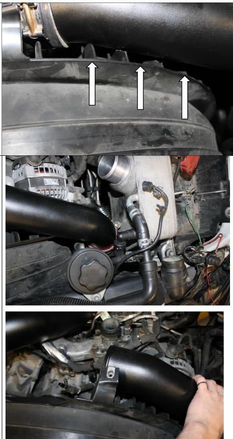
**9.9** Install the 3.5" lower CAC tube as shown. Assure the 3" intercooler joint snaps into place. Do not tighten the clamps until aligned (see photo). The tube should be aligned compared to the fan shroud. The end of the tube should sit almost flush with the tab when lifted forward. All clamps can be tightened until spring is bound.
