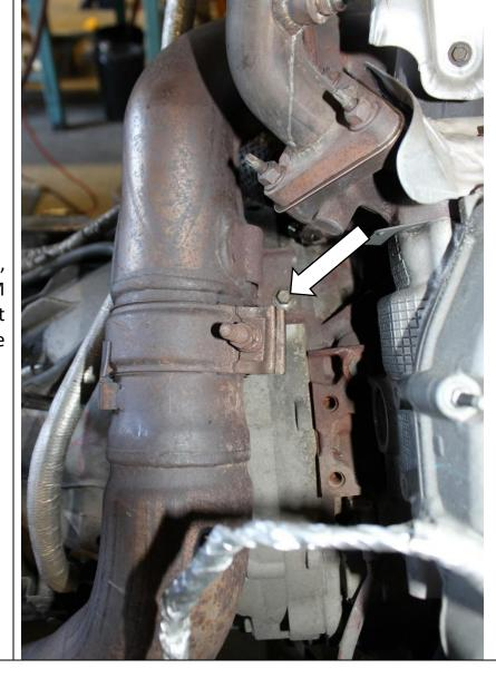
**R3.2** Using a 10mm Socket, remove the bolt holding the OEM cobra downpipe, this is found at between the rear of the engine and the upper down pipe.
