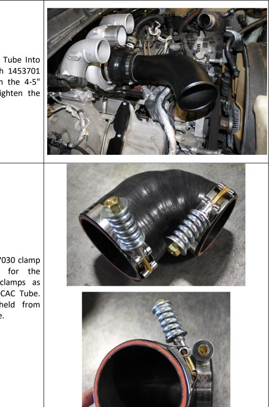
**9.6** Place the 4" Intake Tube Into position as shown, with 1453701 gear clamp installed on the 4-5" intake boot. Do not tighten the gear clamps at this time.
