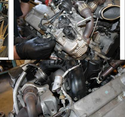
R1.2 Using a 10mm socket & 16mm wrench remove the EBP sensor and tube at located at the rear of the EGR Cooler. Place the sensor and tube aside this will be reused in the BD Install procedures.
