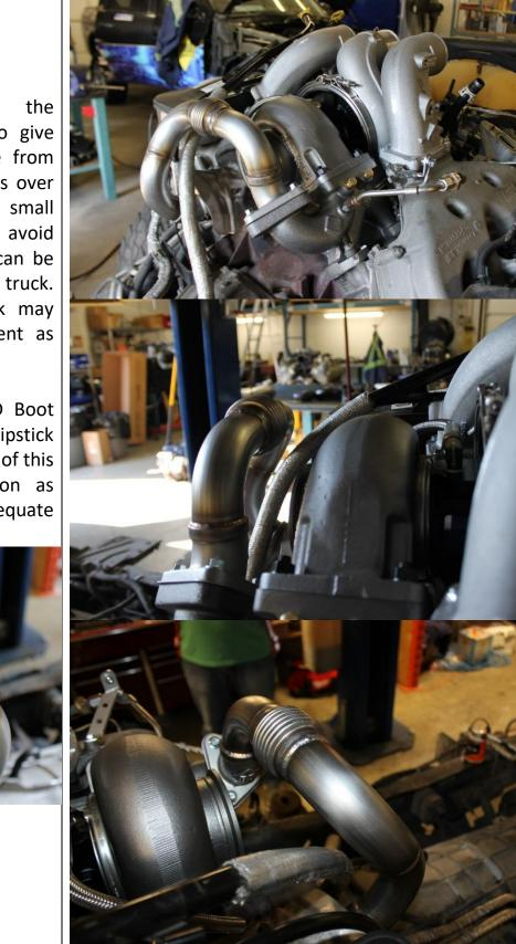
5.4 Carefully bend the transmission dipstick to give 1/2" to 3/4" clearance from the dipstick to the cross over tube as shown. Make small adjustments evenly to avoid kinking the tube. This can be done by hand on the truck. The engine oil dipstick may need a small adjustment as well for best fitment.
