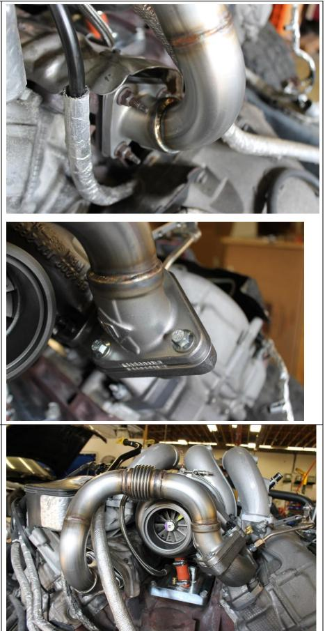
**5.2** During this section assure the transmission dipstick is on the inside or front of the cross over tube. It will need to be massaged into shape to clear in the following step.
