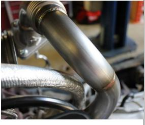
**5.5** Install the 2 1900037 M6 dipstick bolts provided with an 8mm socket and torque to 89 inch lbs.
