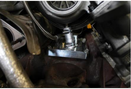
**3.16** Install the oil feed line, take care to assure this line is clear of the driver side manifold, turbine housing and other sources of heat or any edges on which this line could wear on. When tightened in final position the oil feed line should be free from rubbing all other items by 1/2 Inch.
