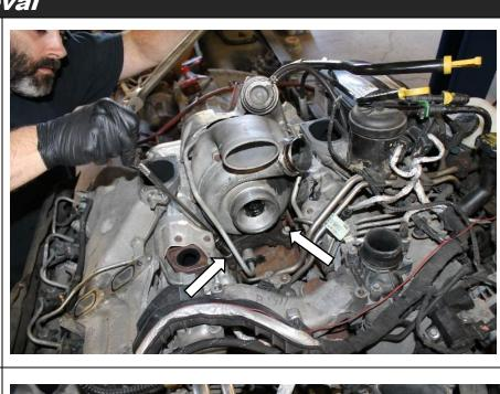
**R4.2** Remove the turbocharger coolant return line found on the driver's side, this simplified by removing the spring clamp on the front of the tube near the coolant cross over in front of the charger. You may also remove the E Clip to allow this tube to be released, this is not required.
