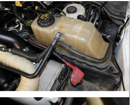
**9.14** Re-install the vacuum and coolant overflow lines into place on the driver's side and the heater line attachment.
