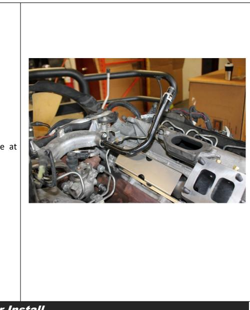
**2.9** Reinstall the coolant tube at this time using a 8mm socket.
