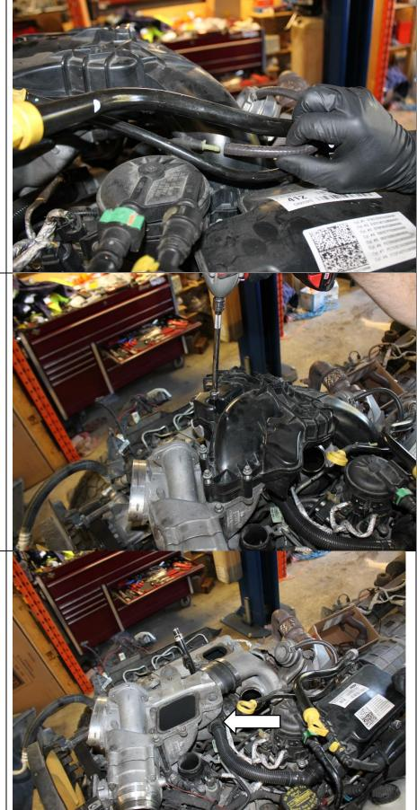
**R2.4** Using an 8mm, socket remove the 15 upper intake bolts. The upper intake can now be removed.
