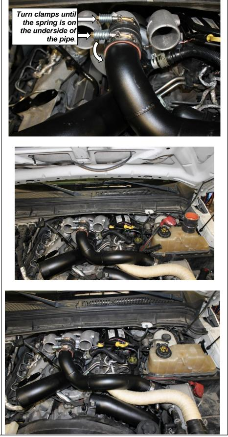
**9.12** Install the 3" Hot side CAC Tube 1403031 with 1401530 boot on turbo with 1405209 and 1405211 clamps. Use 1 3" 1405305 boot and 2 3" 1405211 clamps on the CAC. Place the T Bolts on the bottom side and pointing towards the passenger side. All clamps can be tightened down until spring bound.
