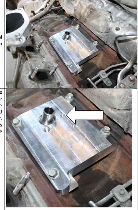
**1.3** Torque down the 4 pedestal block off plate bolts using a 13mm socket to 41 ft. lbs.
