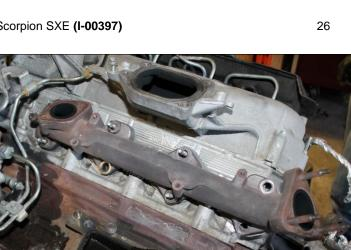
**R.2** Using a 13mm socket, remove the 8 main manifold nuts. Some studs may come with these and will need to be reinstalled after manifold removal. The manifold can now be removed from the passenger side head. If any studs were removed reinstall these and torque to 115 lb-in.
