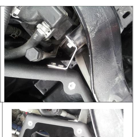
**10.9** Reinstall the radiator screw and air box bracket as shown.
