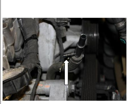
**7.8** Cap the shown location where the wastegate actuator solenoid was fed using the supplied Rubber bullet cap (1900068)
