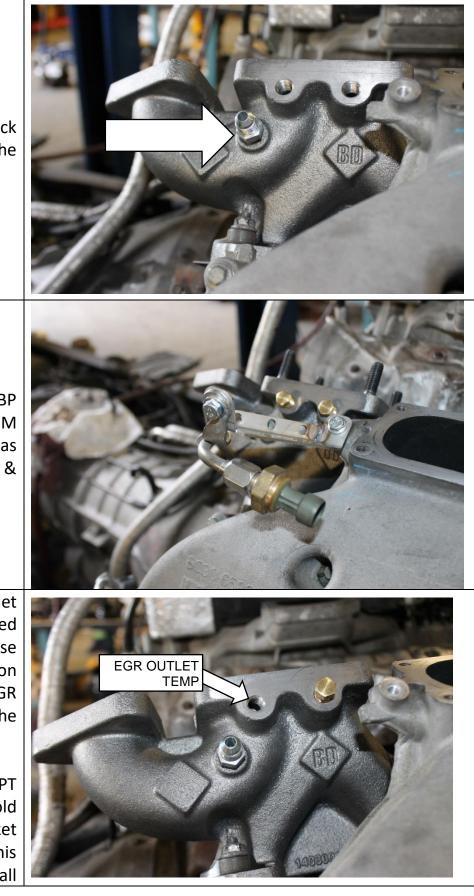
**2.5** Install the (EBP) exhaust back pressure JIC fitting into the manifold (5/16" X -8 JICM).
