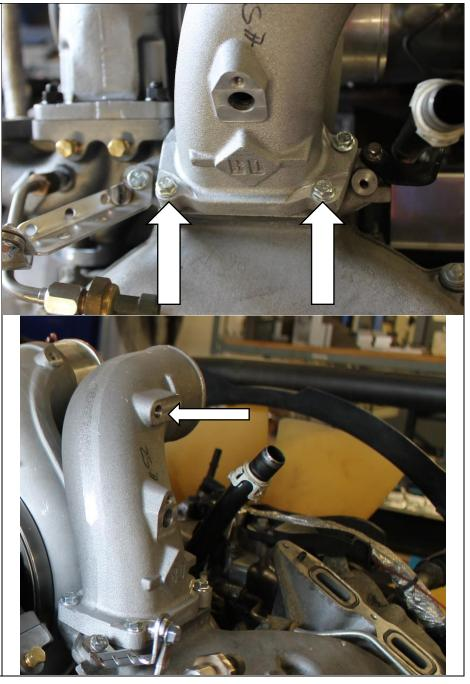
4.3 Repeat the process for the passenger side intake horn, and torque to 89 inch lbs.
