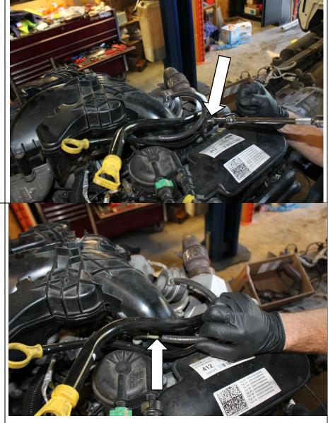
**R2.2** Using an 8mm socket remove the two bolts holding the two dipsticks to the intake on the driver's side.
