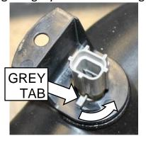
**9.2** Install the OE IAT into the BD CAC Tube 1403032-1. Rotate until the clip locks into place as shown.
