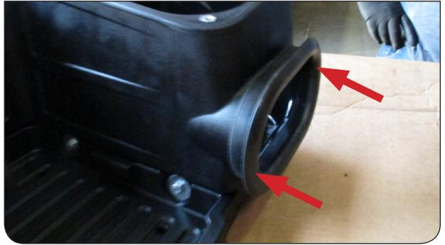
**15** Install the Tube Seal (E) onto the Air Box (O).
