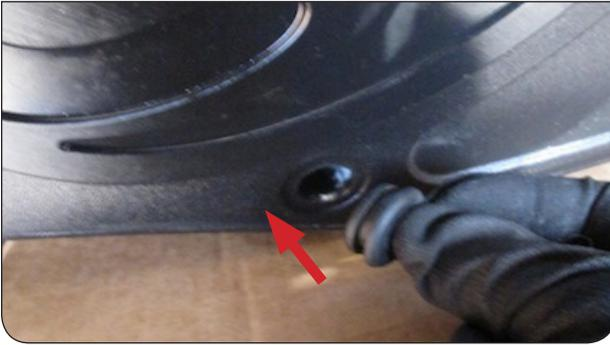
**14** Install the Fender Seal (R) onto the Air Box (O).
