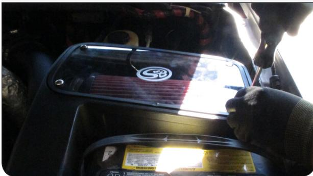
**32** Install the air temperature sensor into Air Box (O) by pushing firmly into the grommet.
