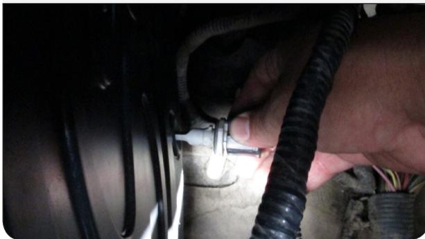
**33** **IF EQUIPPED:** reconnect the electronic restriction gauge and push it into the grommet on the intake tube. Press firmly to ensure a air tight seal.
