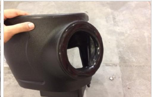
**6. (OPTIONAL)** For those concerned about minimal engine heat; install the Box Plug (K) onto the bottom of the Air Box (A) using the provided 1/4-20 Screws (N), Lock Washers (M), Flat Washers (L) and Locknuts (S). For those seeking additional air flow, set the box plug aside.
