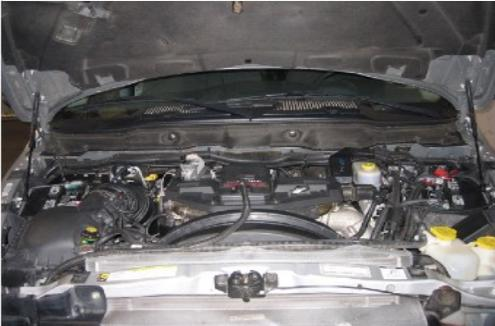
**2.** Disconnect the electrical connection for the Intake Air Temp (IAT) Sensor, then unclip the wire loom from the tube.
