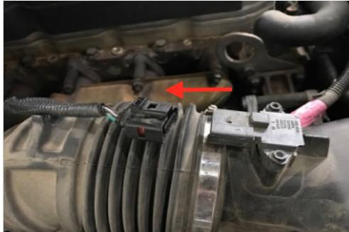
**3.** Loosen the hose clamp connecting the intake tube to the air box lid then remove the mounting nut securing the stock air box. Pull up on the stock air box to remove it from the vehicle.
