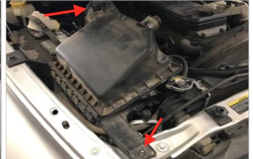
**4.** Loosen the hose clamp at the turbo inlet and then remove the intake tube from the vehicle.
