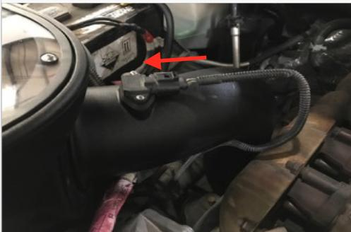
14. Reconnect the negative terminal on both batteries. Inspect your installation, make sure the kit is properly positioned and all fasteners are secure. Affix the CARB and ID label near the intake kit. The installation is now complete.
