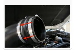
20. Carefully place the Air Filter (E) into the Air Box (A) then slide the air filter onto Intake Tube #1 (D) and rotate the filter so that it points towards the bottom opening of the box. When positioned tighten the #88 Hose Clamp (F). Make sure the filter is not rubbing against the box or touching anything.
