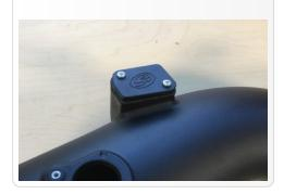
14. For 2013-2016 Models Only. Carefully remove the humidity sensor from the stock air box lid. Install the Gasket (P), the MAF Mount (Q), and humidity sensor onto Intake Tube #2 (K) with the supplied M4 Screws (S)
