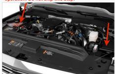
2. Disconnect the electrical connection for the MAF sensor. For 2013-2016 Models, disconnect the electrical connection for the humidity sensor.
