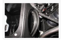
19. Place the two #80 Hose clamps (M) over the Hump Coupler (L) then over Intake Tube #1 (D). Leave the clamps loose for now.
