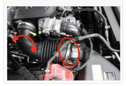
8. Remove air box lid and air filter by removing the two screws by the fender. Then carefully pull the lower portion or the air box up out of the two rubber grommets.
