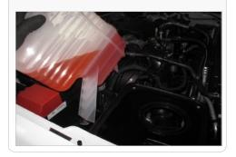
16. Reinstall the coolant reservoir and mounting hardware that was removed in Step #10 & 11
