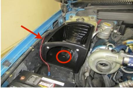
11. Loosely install the Air Box (P) to the wheel liner using the supplied 3/8"x1.0" Button Head Screw (F) and Fender Washer (O) on top and the 3/8" Nylock Nut (N) and Fender Washer (O) in the wheel well.
