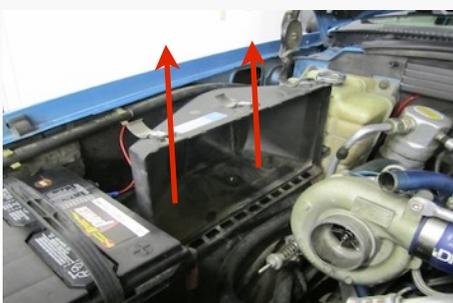
8. Remove the OE snorkel from the fender by pressings in the sides and popping it out towards the motor.
