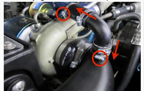
18. Completely loosen the #64 Hose Clamp (E) around the air filter base. Then carefully place the Air Filter (D) (base end first) inside the Air Box (P). Push the base of the filter over the Intake Tube (L) and tighten the hose clamp.
