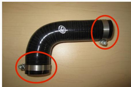
17. With the 2 #16 Hose Clamp (J) in place, slip the longer hose end of the assembly onto the OE vent tube and then push the smaller hose end onto the intake tube. Fully tighten the all hose clamps.
