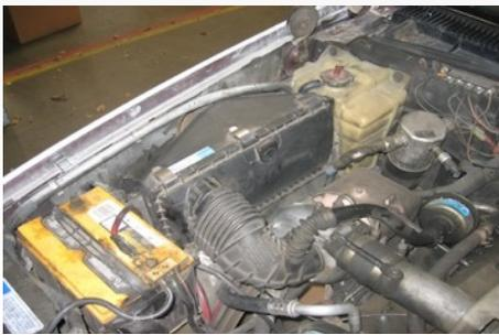
2. Loosen the hose clamp at the turbo.
