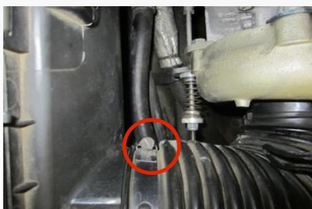
5. Unclip the air box cover from the air box. Remove the cover and filter from the truck.
