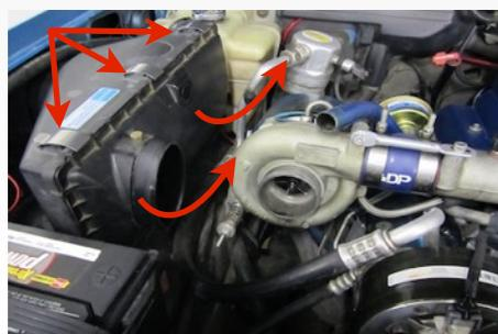
6. From under the wheel well, remove the 2 bolts mounting the air box.
