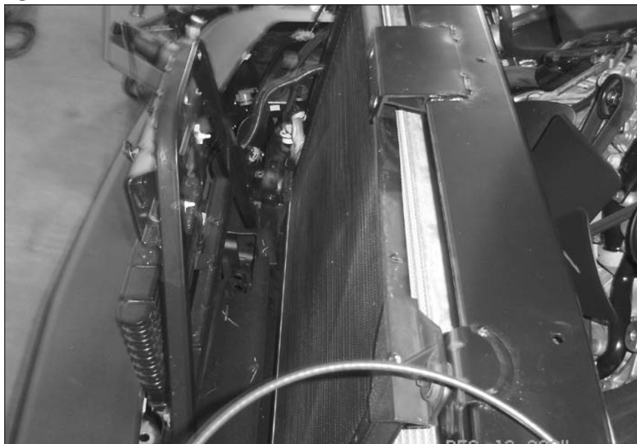
Figure 13 Latch support moved out of the way
