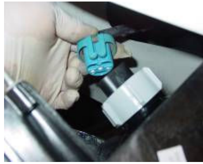
Step 10: Put in the new Anzo light and plug in the headlight harness.
